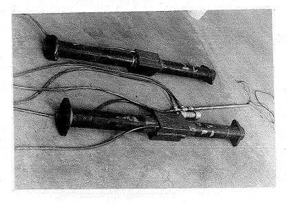
Two test pipes ready for installation with copper sleeves and plastic hoses covering electrical strain gauge leads.
