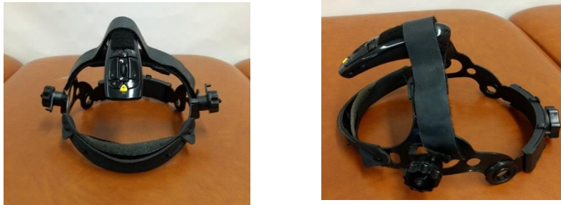
Figure 1: Wireless scoop pointer air mouse from Hilcrest Lab (Rockville, MD) mounted on Helmet worn by participants
