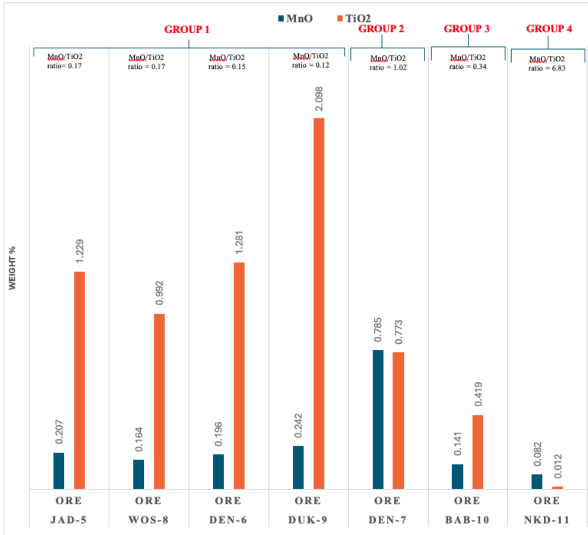
Figure 4.8: MnO and TiO 2 concentrations (ppm) of ore samples and the corresponding MnO/TiO 2 ratios showing four major groupings. (Source: Author)
