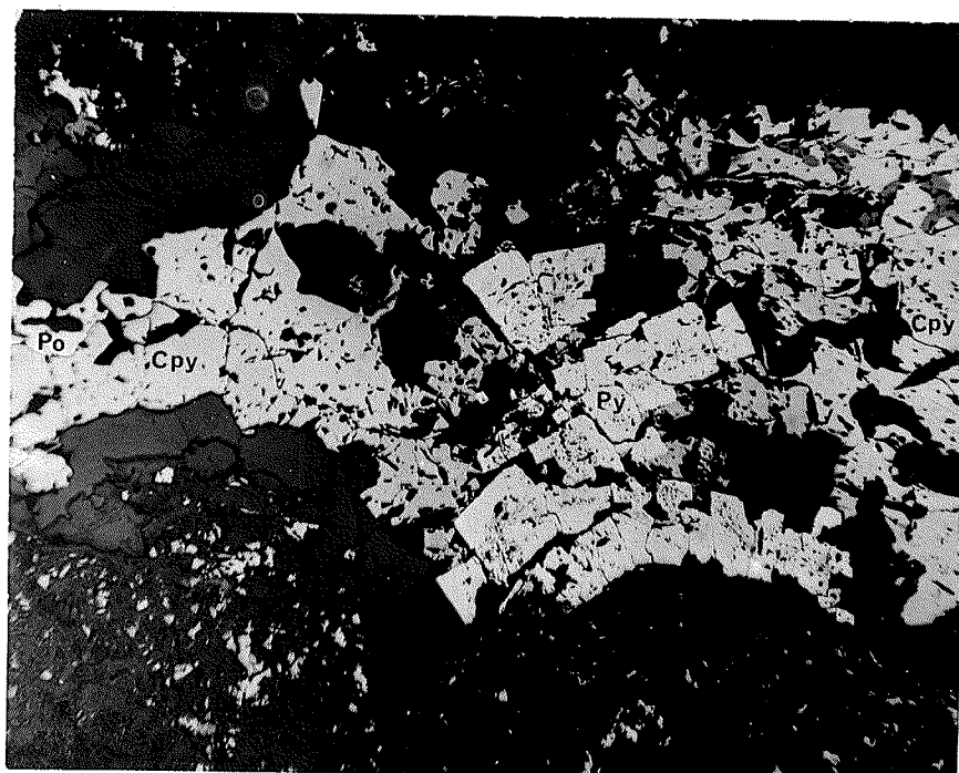
Plate 27 Pyrite, pyrrhotite and chalcopyrite in a sulphide vein within the disseminated sulphides C73 31X
