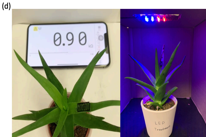
Figure 5.11 The ultra-thin plant growth sensor. (a) The aloe leaves growth rate in 18 days; (b) Photo images of the ultra-thin wearable sensor; (c) The resistance of ultra-thin plant wearable sensor during aloe leaves growth in 18 days; (d) Photos of ultra-thin wireless sensor on aloe leaves (control group) and aloe plant with LED light treatment group.
