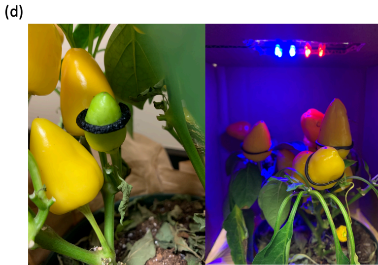
Figure 5.13 The elastic band growth sensor for pepper plants. (a) The percentage of pepper growth; (b) Pictures of elastic band growth sensor on control group; (c) The resistance of elastic band pepper plant growth sensors; (d) Photo images of elastic pepper fruits growth sensors on LED light treatment group.
