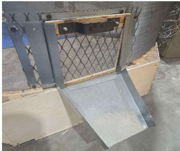
Figure 6. Side door assembly.
