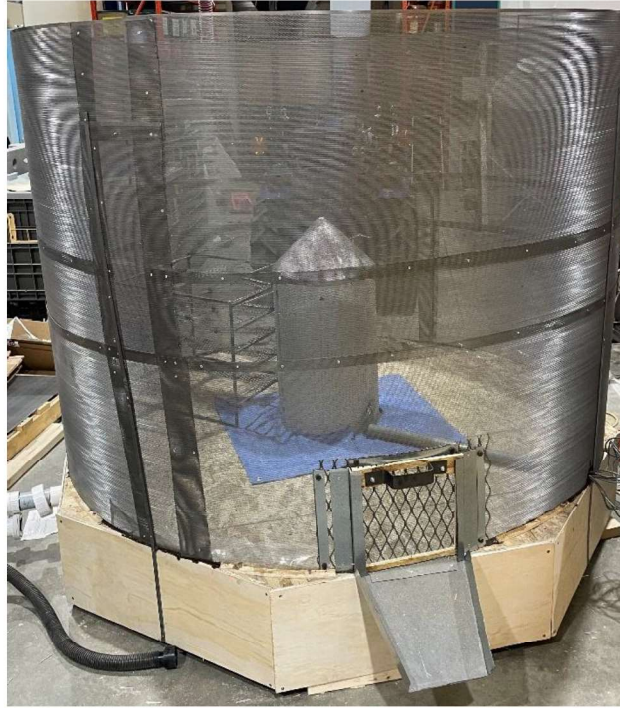
Figure 5. Concentric perforated columns and side door.
