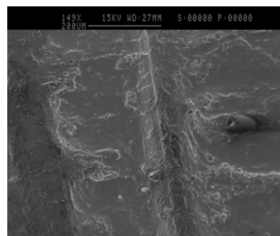
Figure 7.8. SEM micrograph of slice mark of sample 16. Photo: Eleuterio Sousa
