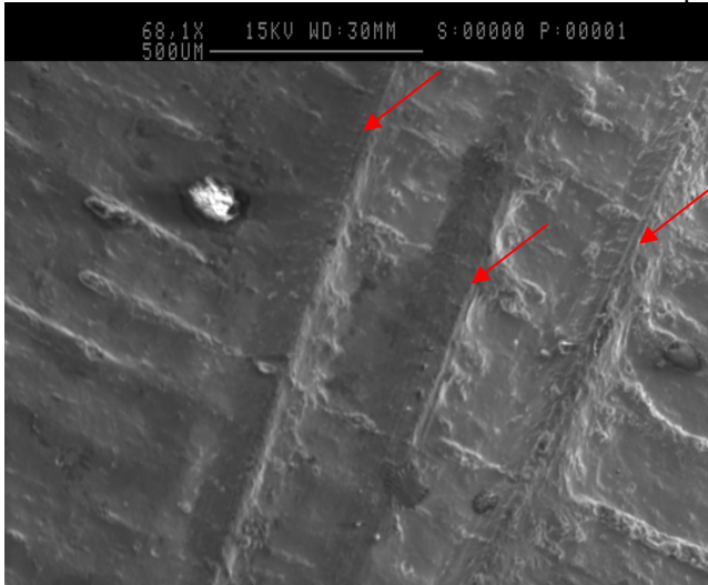
Fig. B. SEM micrograph of slice marks. A. 500 \mu aerial angle. A clear V shape is seen in all three slices with striations (red arrow) characteristic of stone tool-type and multiple slices.
