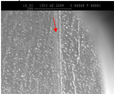
Fig. E. SEM micrograph of slice mark. A. 2mm aerial angle. The striations (along the red arrow) characteristic of stone is visible.
