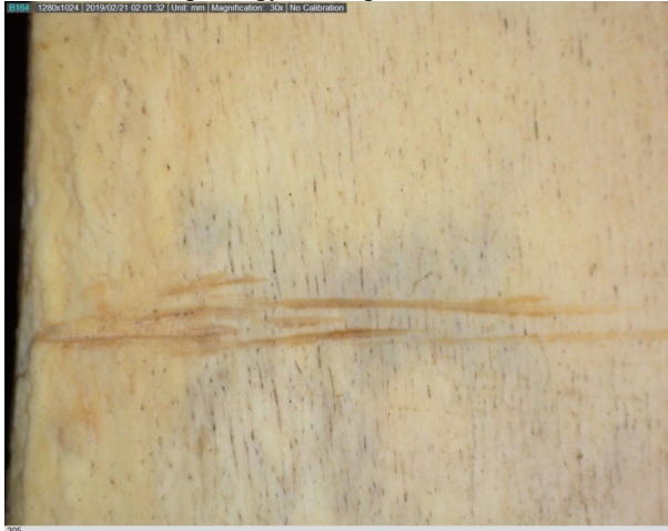
Figs. A-B. Dino-Lite microscopy of multiple slice marks. A. 30x magnification aerial angle. B. 220x magnification. You can see what appears to be a clear, deep, V shape characteristic of metal.
