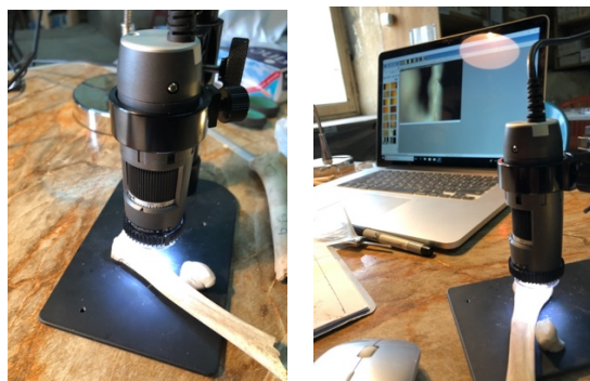
Figure 7.3. Dino-Lite AM4115ZT USB microscope camera with polarizer. Photo: Eleuterio Sousa
