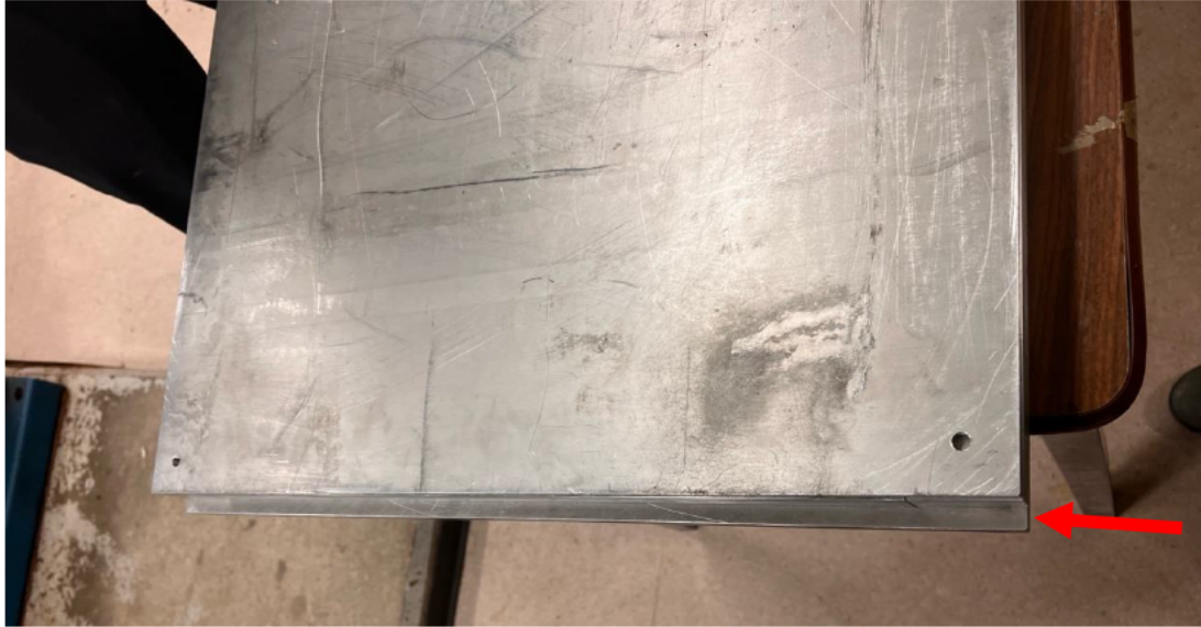
Figure 7. Mistake made in manufacturing of mold.
