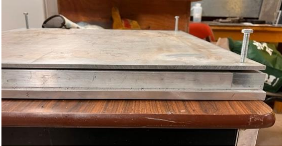
Figure 19. 3/8" - 16 thread bolts to release mold.
