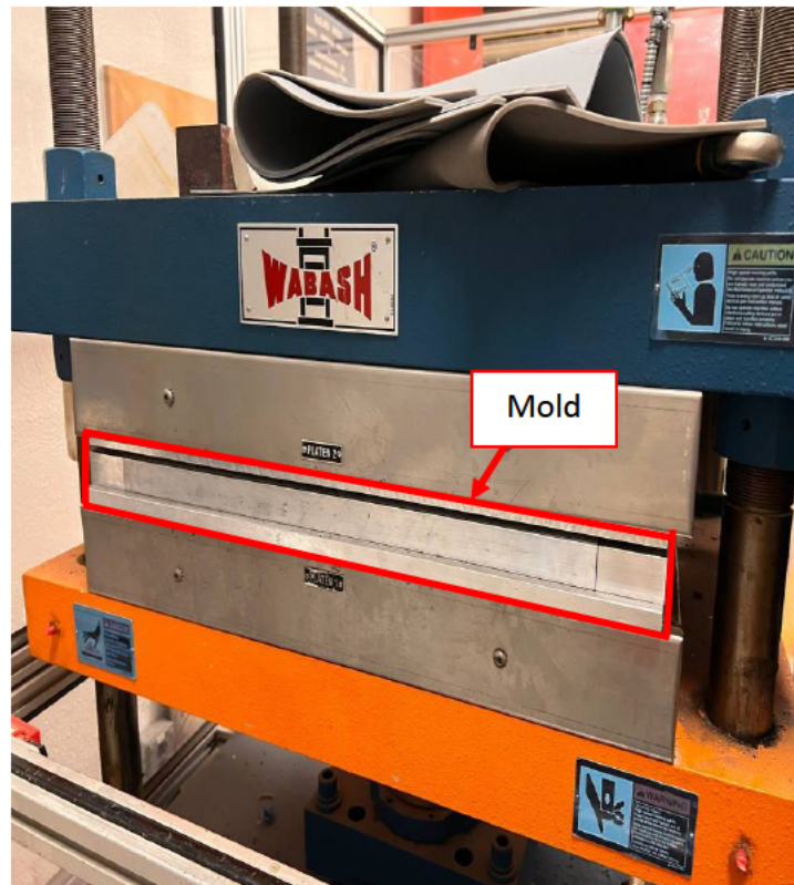
Figure 15. Wabash Hydraulic Press with Shingle mold inside being compressed
