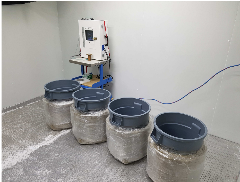
Fig. 5.8: Four insulated containers used to grow ice from water having different salinity. The containers were approximately 60 cm in diameter, with a water depth of 18 cm. This experiment was performed at a cold laboratory located in CEOS.
