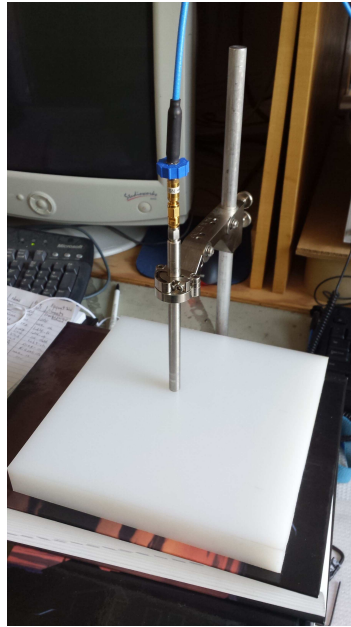
Fig. 4.3: Experimental setup for determining the complex permittivity of the UHMW plastic using a high performance probe.
