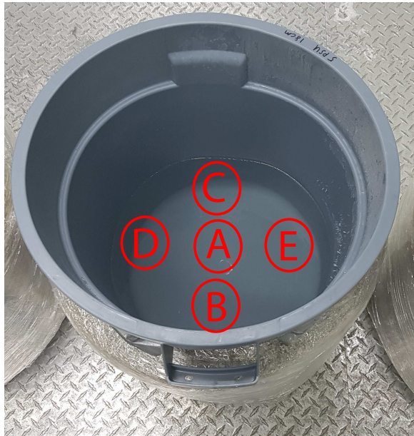
Fig. 5.10: The |S_{11}| measurement locations. At each location two measurements were taken orthogonal to one another.
