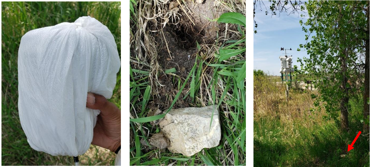
Figure 4. Left – shows container wrapped in plastic, middle – shows hole that will fit the container and rock used to cover it, right – red arrow indicates location of rock where the eggs are buried for house 1 at OHM.
