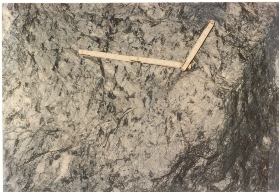
Plate 43: Altered diabase sill or dike margin (Unit 6). Anthophyllite asterisms in matrix of cummingtonite and plagioclase. Location: 2800 Level - 70670E x 10690N.
