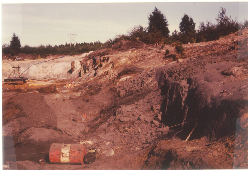
Plate 49: Fault surface defining southern ore contact. Slickensides indicate downward movement of the hanging-wall block (left in photo). Viewed from northwest. Location - 70800E x 9600N.
