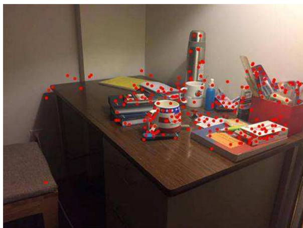
Figure 2.4: Keypoints detected with SURF
