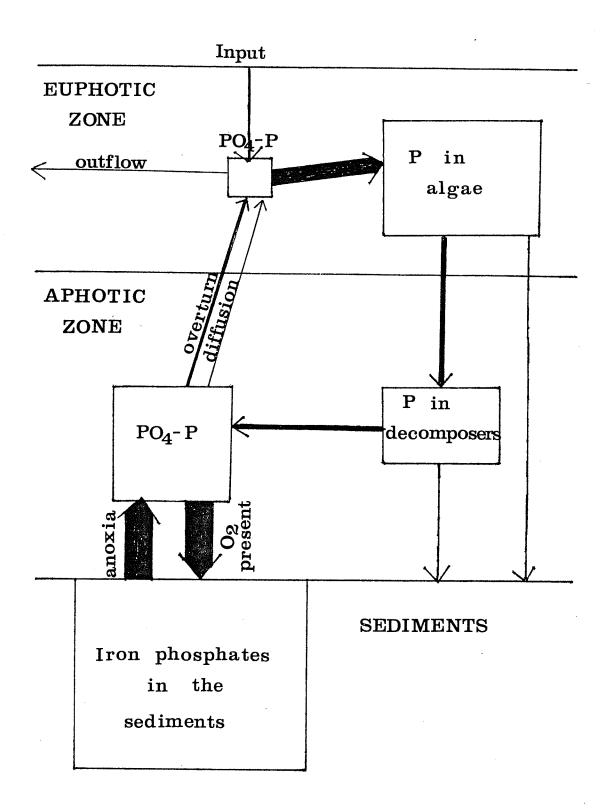
Figure 9. Lean's model of the phosphorus cycle within the epilimnion.
