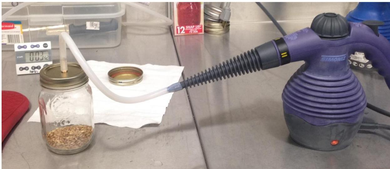
Figure 3.2 Steaming apparatus used in conditioning heat treatment
