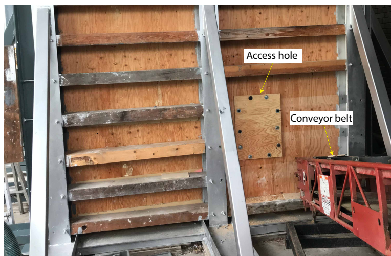
FIGURE C.2: Test preparation: access hole and conveyor belt
