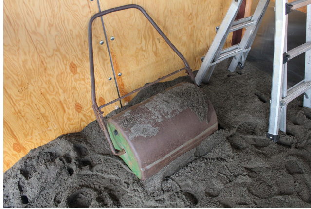
FIGURE C.13: Test preparation: 100-kg static roller
