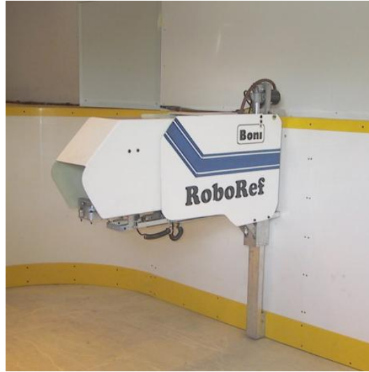
Figure 32: The RoboRef puck dropping machine mounted to hockey rink boards [1].
