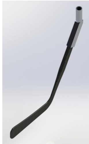
Figure 21: Collar holding the hockey stick [26].
