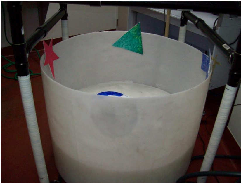
Figure 4. The Morris water maze apparatus. The photo shows the tank used for the Morris water maze experiments with the attached visual cues. The animal use these visual cues to assist with orientation as it attempts to locate the hidden the platform.
