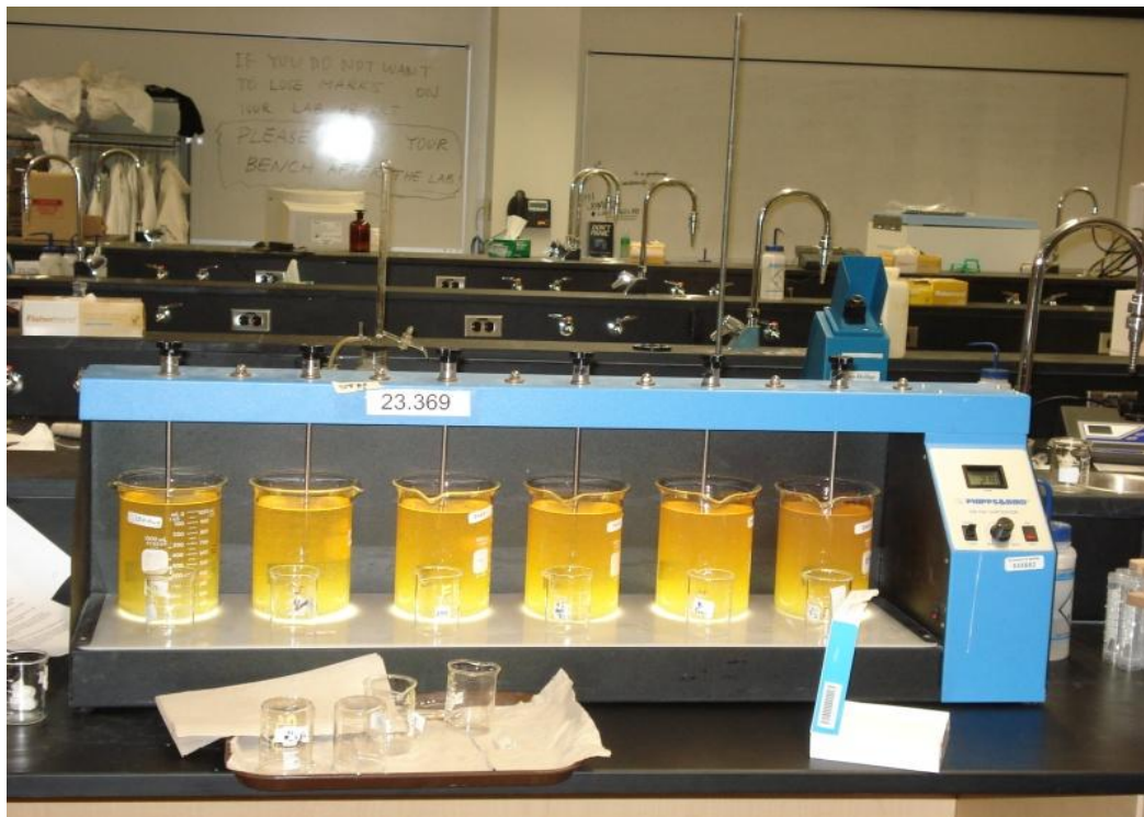
Figure 3 Jar testing apparatus used in this study
