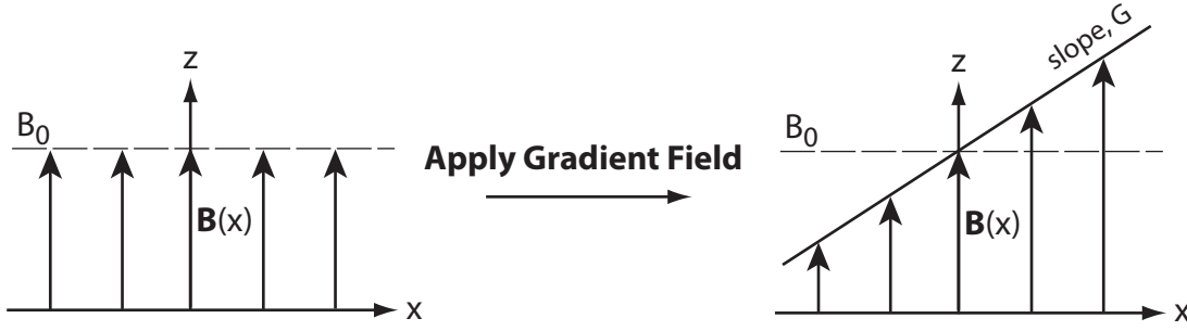
Figure 2.7: Spatially-independent magnetic field, \mathbf{B} = B_0\hat{\mathbf{z}} (left) and spatially-dependent magnetic field, \mathbf{B}_z(x) = (B_0 + G_x x)\hat{\mathbf{z}} (right).
