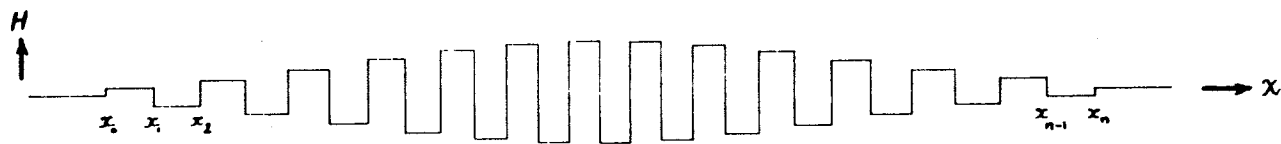
FIG. 3.1 GEOMETRY OF THE UNDULATED CONDUCTOR USING DESIGN EQUATIONS
