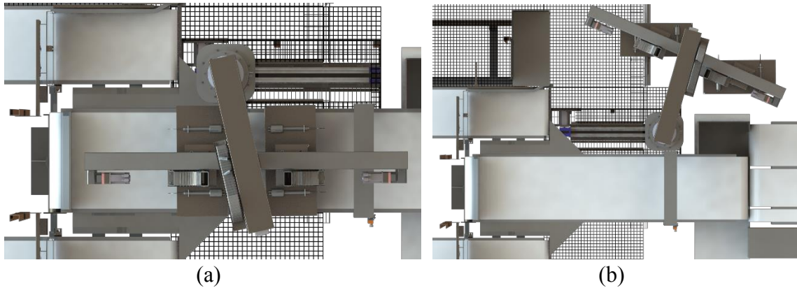
Figure 20. a) The illustration of the feeder when it is at the ' automated ' mode b) The illustration of the feeder when it is at the ' manual ' mode
