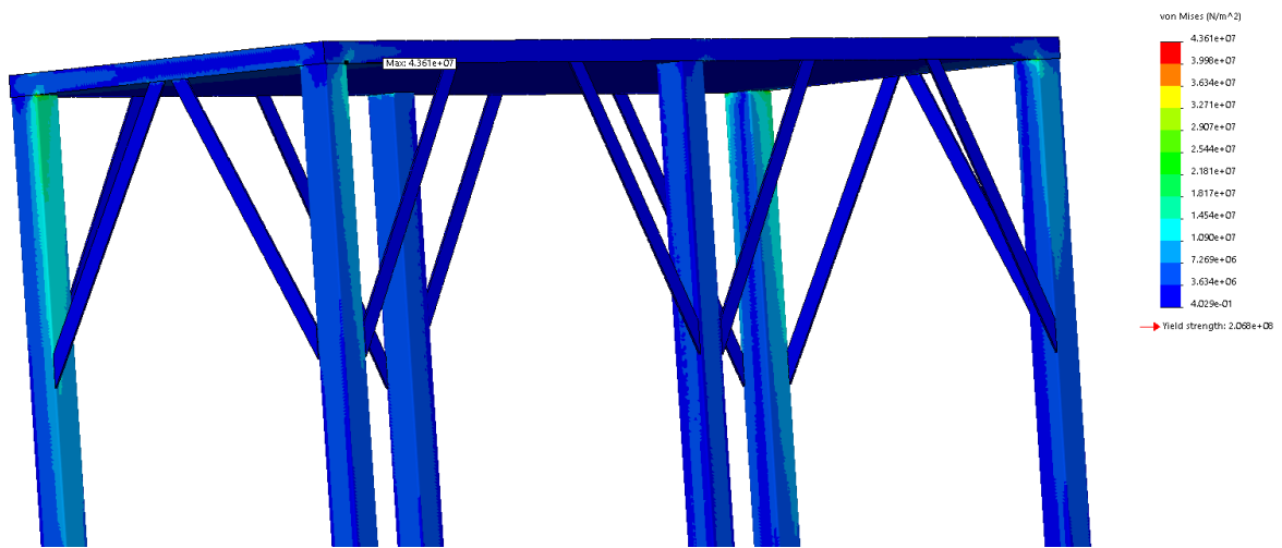
Figure A55. Close-up view of the stress results for the simulated arm base truss support
