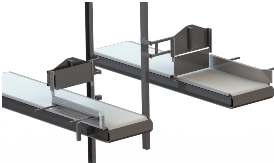
Figure 27. Up and down positions of the gates
