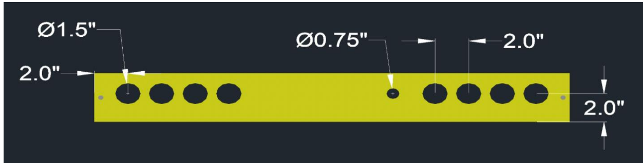
Figure 9. Dimensions for ventilation and wiring holes
