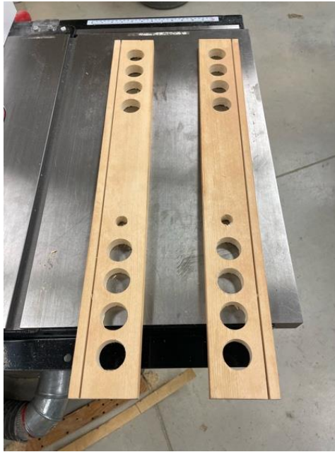
Figure 21. Cut side pieces for the frame
