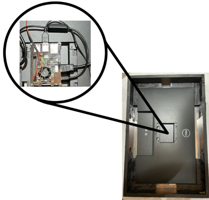
Figure 12. Raspberry Pi secured in the back of the monitor
