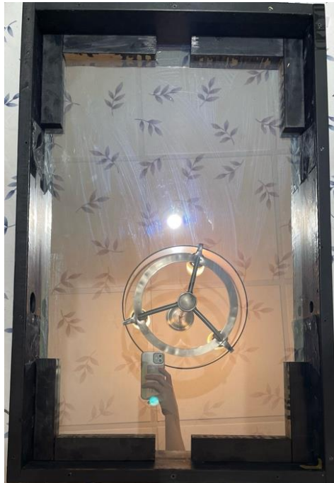
Figure 25. Placement of the corner support pieces
