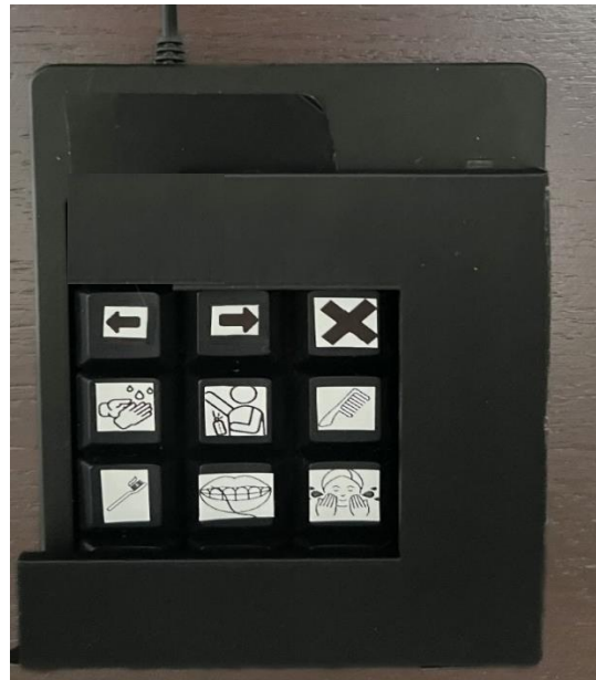
Figure 15. Modified Insignia keypad with 3D-printed cover and icons representing the tasks described in Table 3
