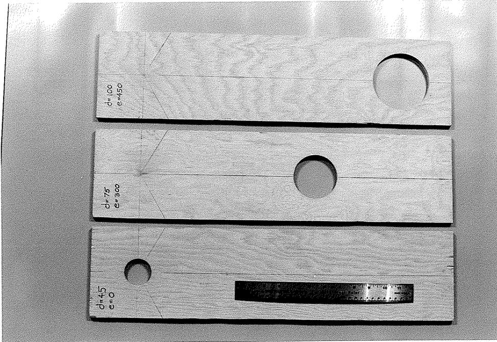
Figure 3.3 - Typical discharge plates
