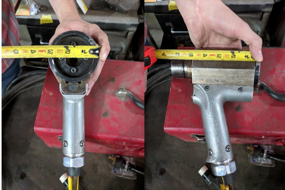
Figure 17. Dimensions of the hydraulic gun used by Cancade.
