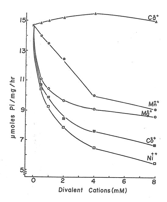
Effect of divalent cations on ATP hydrolysis by dog heart membranes in the presence of 8 mM Ca<sup>++</sup>. The assay system was the same as in the Methods except that varying concentrations of different cations, Ca<sup>++</sup> ((a), Mn<sup>++</sup> ((a)), Mg<sup>++</sup> ((a)), Co<sup>++</sup> ((a)), and Ni<sup>++</sup> ((a)) were also present in addition to 8 mM Ca<sup>++</sup>.
