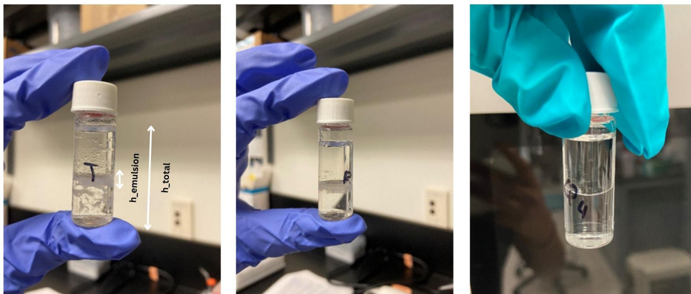
Figure 4.S. 3: Emulsification index ( E_{24\%} ) test of cell-free supernatants from enrichment cultures CMO_MOS_T and CMO_MOS_R grown at 4 °C, and CMO_MOS_Q4 grown at 20 °C, demonstrating their ability to form stable emulsions. Visible emulsification was observed in cultures CMO_MOS_T and CMO_MOS_R, whereas CMO_MOS_Q4 showed no detectable emulsification after 24 h.
