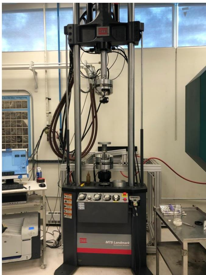
**Figure 5.11 Testing machine linked to computer**
