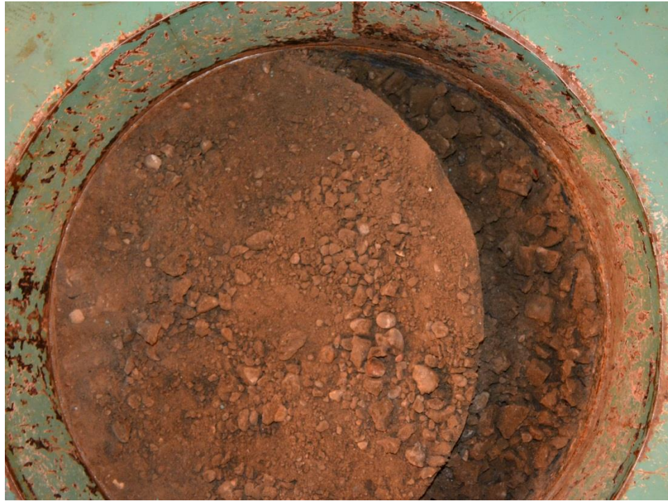
Fig. 3.7. Observed chunks within shear plane after frozen direct shear tests.
