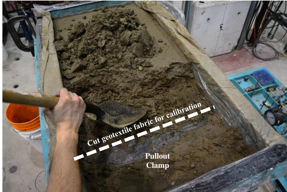
Fig. 4.6. Excavation of soil and cutting of geotextile after pullout test for calibration tests.
