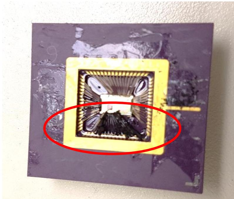
*Fig. 3.7 Undesired polymer growth on the wire bonds exposed to the electrolytic solution*
