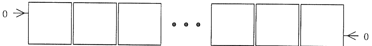
Figure 5.2b): One-dimensional CA with Null boundary conditions.
