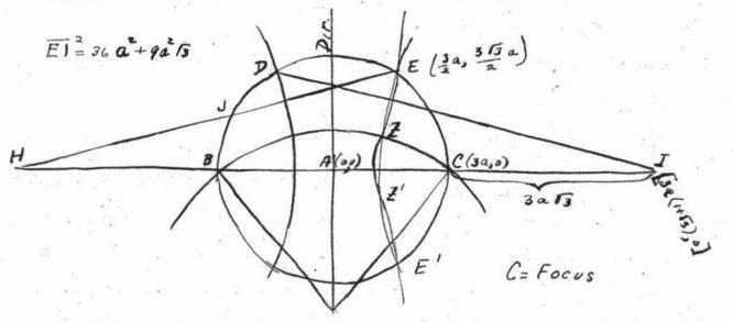
The circle and hyperbola cannot intersect in more than four points, of which two are E and E'. The other two Z and Z'lie between these. The construction works for these points only though it is very close for its whole length.
