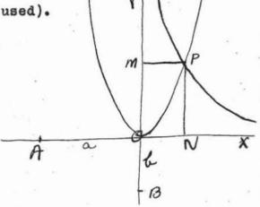
Construct a parabola with b as latus rectum and OY as principal axis, so that its equation is  $\begin{array}{c} 2\\ x\\ \end{array}$  = by and the hyperbola such that the rectangle formed by the perpendiculars drawn to the
