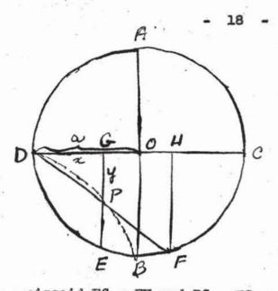
AB and CD are diameters of the circle perpendicular to each other and G and H are points equidistant from the centre. GE and HF are perpendiculars to DC. Join FD and the cissoid is the locus of points of intersection of DF and GE for all positions of G (and of H). In the cissoid EG = FH and DG = HC so that  $\frac{CG}{GE}$  =  $\frac{DH}{HF}$  and  $\frac{CG}{GE}$  =  $\frac{GE}{DG}$
