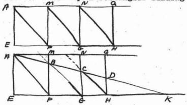
Let AE and DH be the given lengths between which it is required to find the two mean proportionals. Slide one rectangle under the other until the straight line joining A and D passes through
