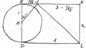
A circle of radius11, having DL and BK tangents of length 3 is drawn. The angle BAJ is constructed to be 30° and JL is joined. Then  $JL = \sqrt{\left(3 - \frac{1}{f_3}\right)^2 + 4} = \sqrt{\frac{40}{3}} - \sqrt{12} = 3.141533$
