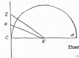
Let the circle have diameter AC with centre E. Let ZEC be one third of a right angle with Z lying on the tangent at C. Then EZ = 2ZC , EC<sup>2</sup> = 3ZC<sup>2</sup>
