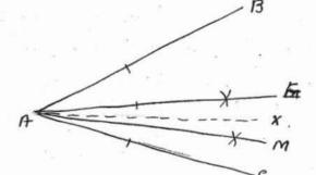
the bisecting lines can no longer be distinguished, and to all intents and purposes XAC is an angle one third the size of BAC. This is actually the sum of the
