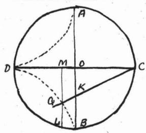
K is taken on OB so that  $\frac{OK}{OC} = \frac{b}{a}(here \frac{1}{2})$ Join CK and produce it to cut the cissoid in Q. Through Q draw the ordinate LM.
