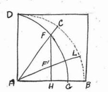
DFG is the quadratix and CAB the given angle which intersects the quadratix at F. Draw FH perpendicular to AB and divide it in the ratio 1 : 2 (or in any given ratio). Join AF'L and LAB is one third of the given angle
