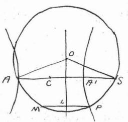
On AS describe a segment to contain the given angle and let the right bisector of AS cut the segment in O. With O as centre and radius OA describe a circle to cut the hyperbola in P. Then the angle SOP is one third the angle SOA. From the definition
