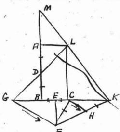
BC and AB are the two given lengths. Complete the rectangle and bisect AB at D and BC at E. Join LD and produce to G on CB produced. Draw EF perpendicular to BC and of such a length that FC = AD. Join FG. Draw CH parallel to FG, having if of such a length that HK = AD
