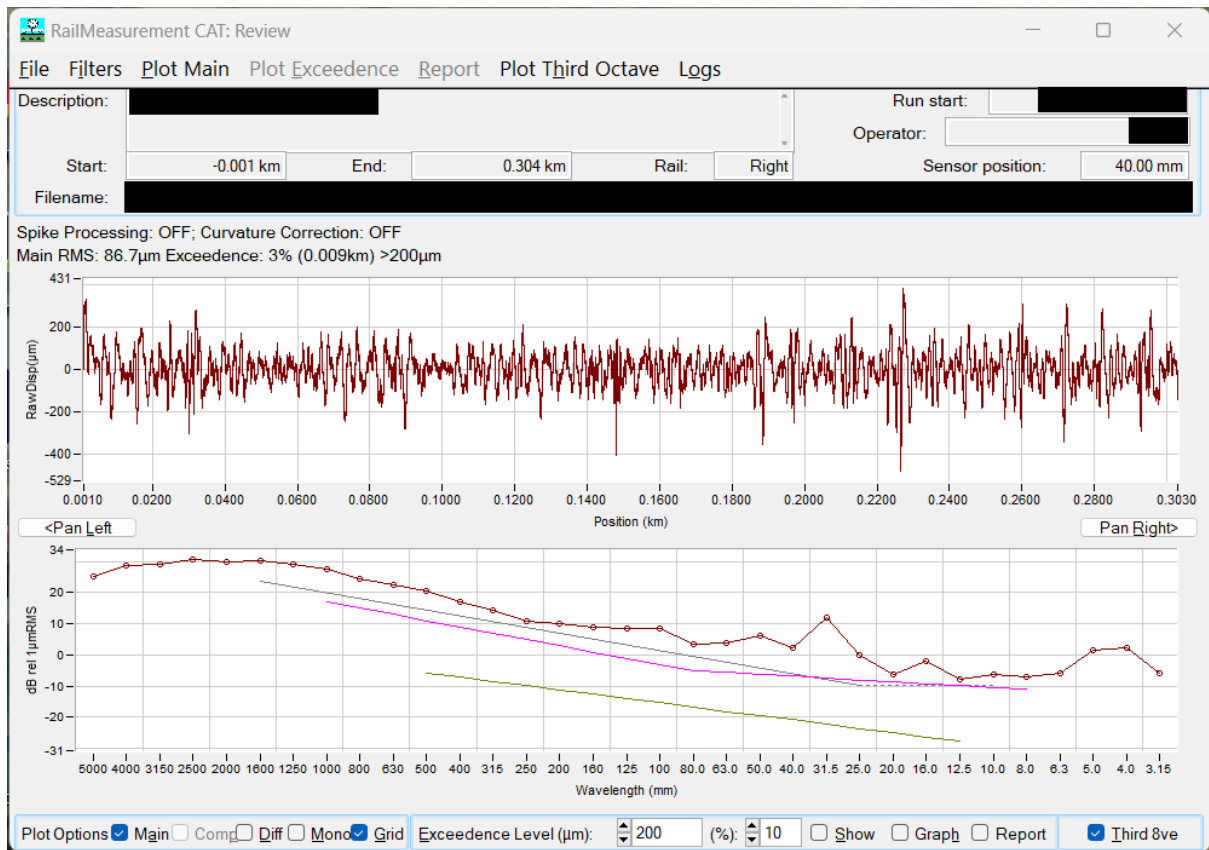
Figure 2.3: Screenshot of RailMeasurement CAT software Version 14.26.21606 visualizing an unfiltered corrugation measurement and the calculated 1/3 octave spectrum of the data.
