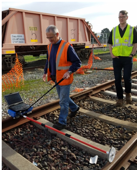
Figure 2.2: Operator logging vertical displacement on the far rail face using the original CAT. The blue box on which the laptop is resting contains the sensor hardware.
