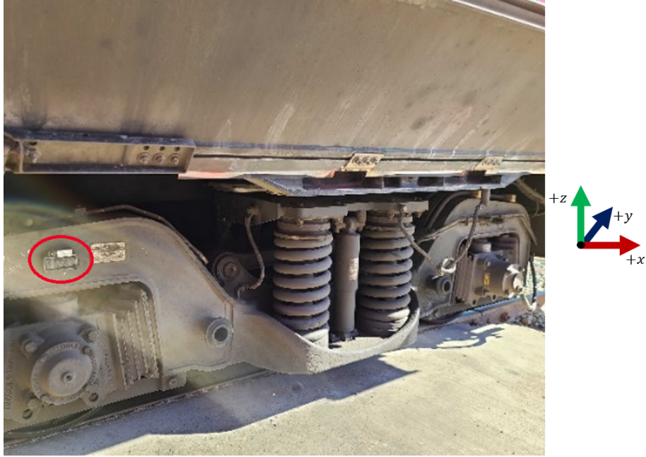
Figure 2.7: ABA mounted on a vehicle, with the IMU's frame of reference.
