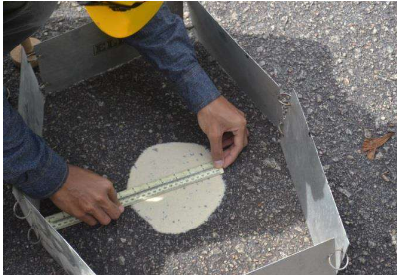
Figure 2.2: Sand patch method to measure macrotexture depth (Yaacoba et al., 2014).
