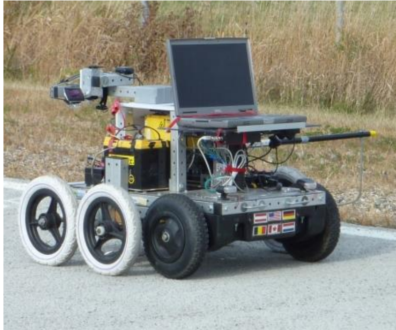
Figure 2.8: RoboTex texture measurement system (Rasmussen, 2010).
