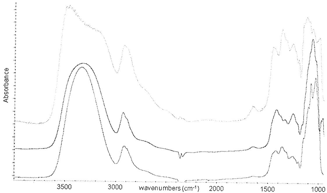
Figure 14 – Infrared spectra of different sugars. Dextrose (red), mannose (purple), and glucose (green).
