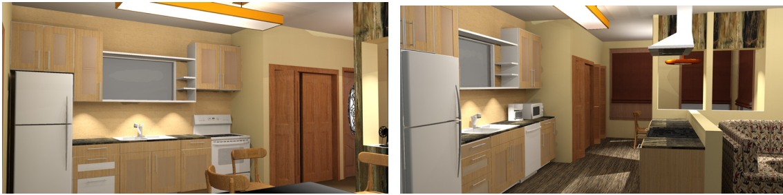
Figure 163: Single Wall Kitchen in Transitional House Transforms to Galley Style Kitchen with Addition of Island in Permanent House. Image by Author.
