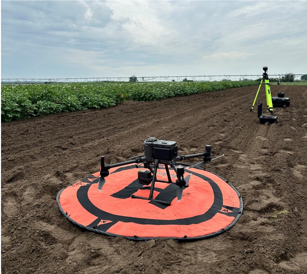
Appendix Figure A1. DJI Matrice 300 RTK UAV equipped with the Zenmuse L1 sensor prior to data acquisition in the experimental potato field; the RTK survey setup is visible in the background.
