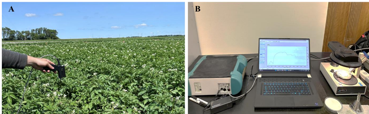
Figure 4.1. Hyperspectral reflectance data acquisition under field and laboratory conditions. (A) Canopy-level field measurements conducted under natural illumination. (B) Laboratory spectroscopy setup for leaf sample measurements under controlled illumination.
