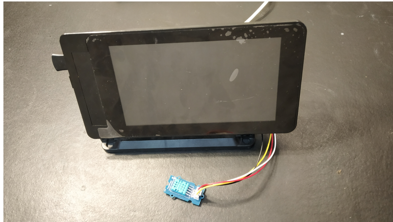
Figure 4.2: Prototype for Measuring Temperature and Humidity
