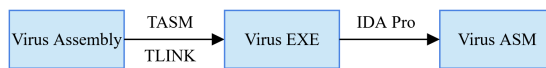
Figure 2.9: Assembly and compilation of a virus executable. Retrieved from personal work in [60].
