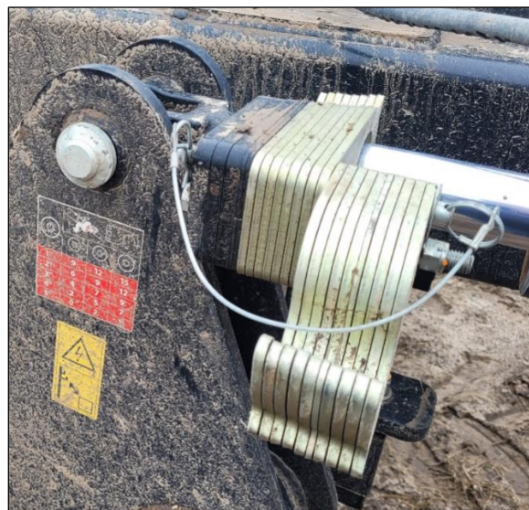
Figure 3.4: Depth stop plates on the hitch of HSCD implement
