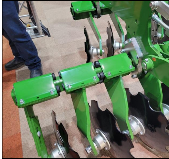
Figure 2.4: Individual disc mounting on Amazone CATROS 03-2TX disc harrow with rubber shock absorbers
