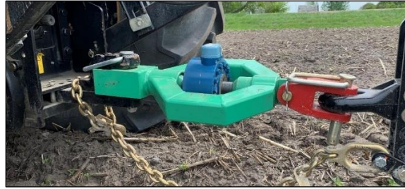
Figure 3.11: Load cell connection to the power unit and the implement
