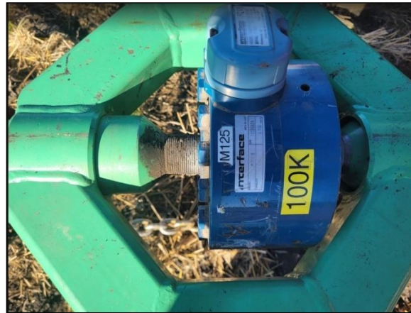
Figure 3.10: Load cell used to collect the draft force data
