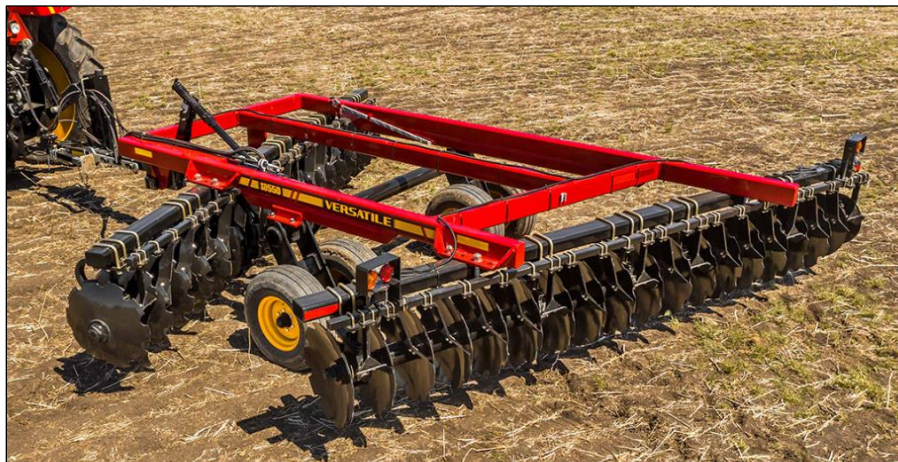
Figure 2.5: SD550 offset disc by Versatile with gangs of notched discs
