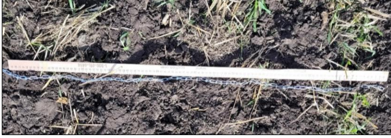
Figure 3.14: Soil surface roughness measurement using the chain method
