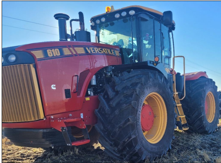
Figure 3.5: Tractor (Versatile 610, 610 hp) used to pull the tillage implement in the experiment
