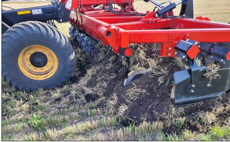
Figure 4.1: Disc harrow dragging soil instead of effectively tilling it
