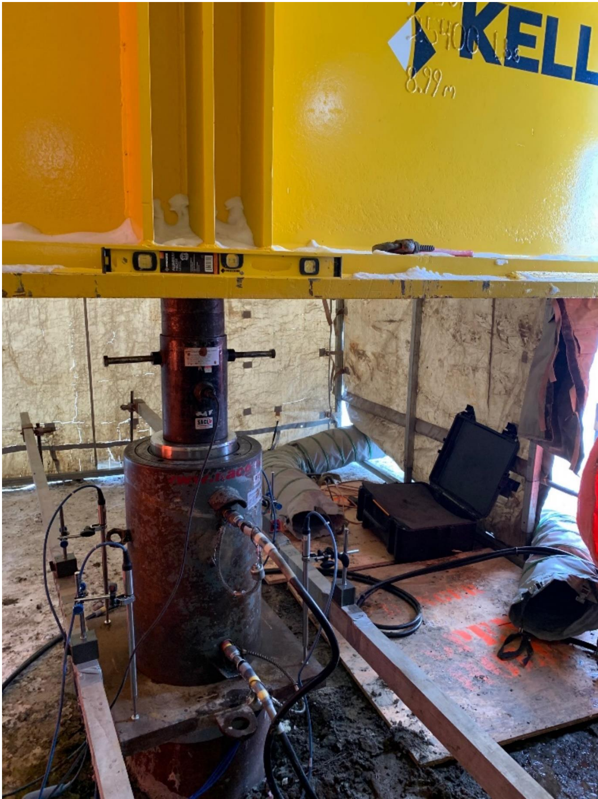
Figure 2.7. Hydraulic jack, load cell, steel test plate, test beam, and test pile
