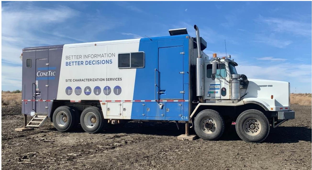
Figure 2.2. Truck mounted CPTu unit
