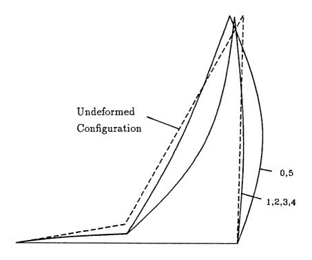
Figure 3.24: Third mode shape,  $\theta=10^{\circ}, \Omega=1000 \text{ rad/sec}$
