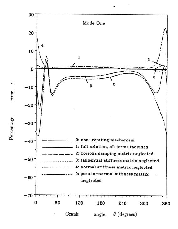
Figure 3.18: Percentage error in natural frequency vs. crank angle,  $\Omega{=}1000\,\mathrm{rad/sec}$
