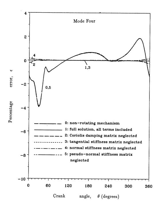
Figure 3.21: Percentage error in natural frequency vs. crank angle,  $\Omega$ =1000 rad/sec
