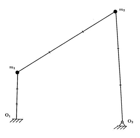
Figure 3.1: Finite element model 3 for the crank rocker mechanism[25]
