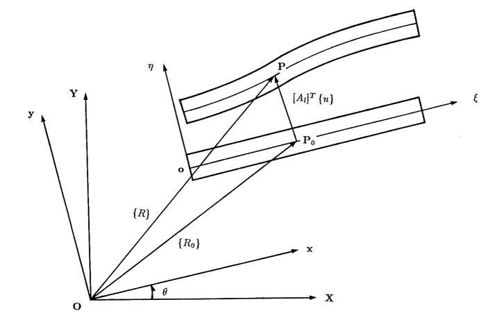
Figure 2.1: A general beam element at the undeformed and deformed configurations depicted in the associated coordinate systems
