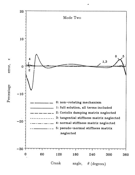
Figure 3.15: Percentage error in natural frequency vs. crank angle,  $\Omega = 500$  rad/sec
