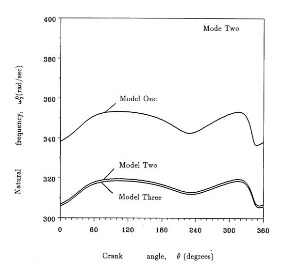
Figure 3.3: Natural frequency vs. crank angle
