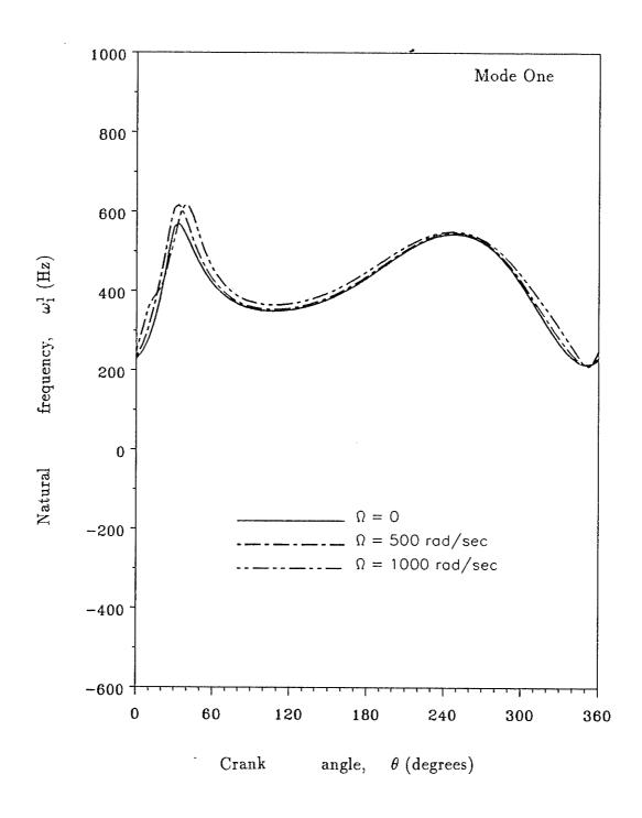
Figure 3.6: Natural frequency vs. crank angle
