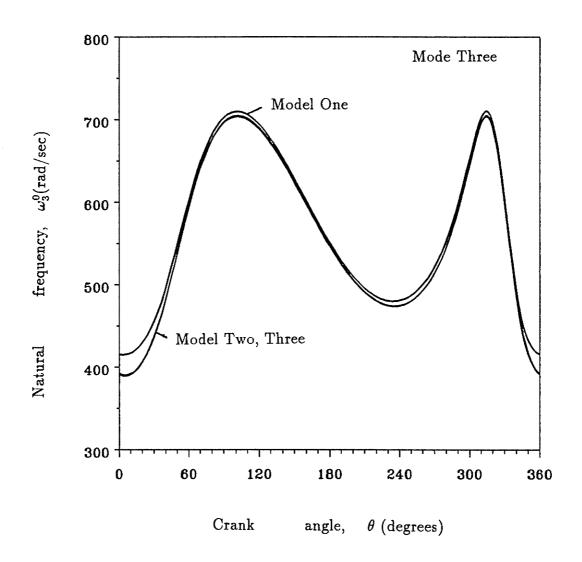
Figure 3.4: Natural frequency vs. crank angle
