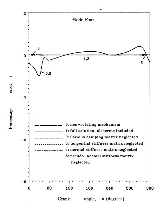
Figure 3.17: Percentage error in natural frequency vs. crank angle,  $\Omega = 500$  rad/sec
