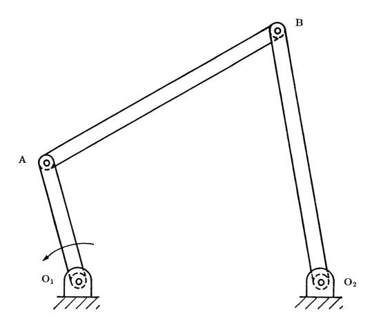
Figure 3.5: A general crank rocker mechanism [15]
