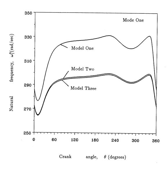
Figure 3.2: Natural frequency vs. crank angle
