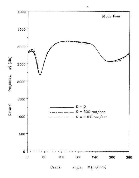
Figure 3.9: Natural frequency vs. crank angle
