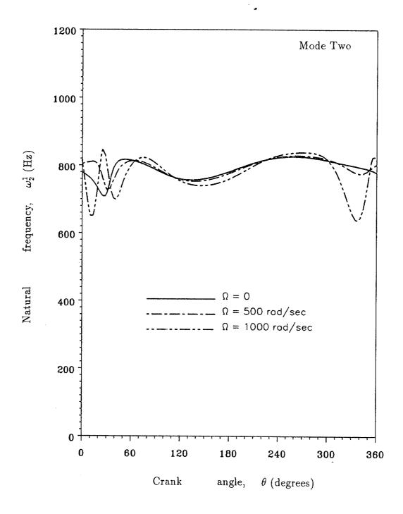
Figure 3.7: Natural frequency vs. crank angle
