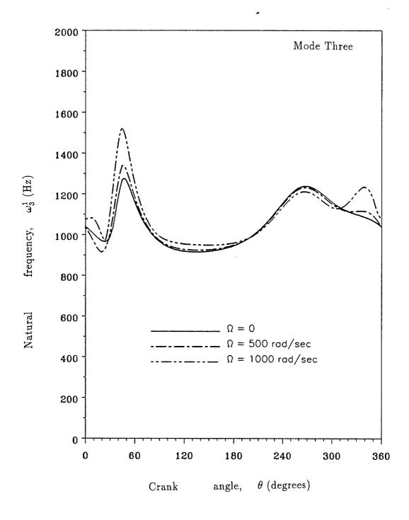
Figure 3.8: Natural frequency vs. crank angle
