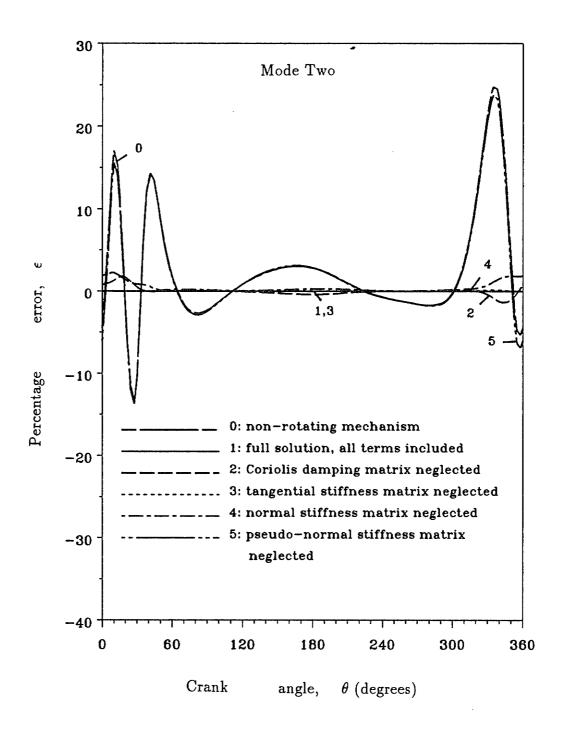
Figure 3.19: Percentage error in natural frequency vs. crank angle,  $\Omega$ =1000 rad/sec
