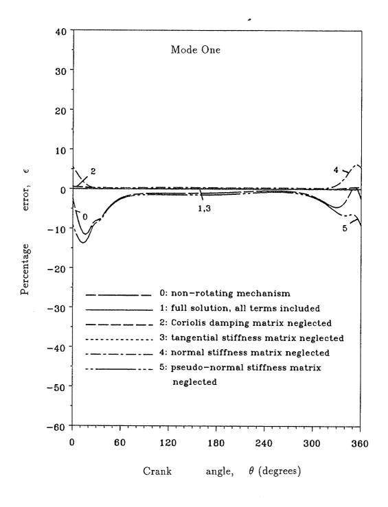
Figure 3.14: Percentage error in natural frequency vs. crank angle,  $\Omega$ =500 rad/sec
