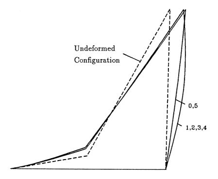
Figure 3.22: Fundamental mode shape,  $\theta=10^{\circ}, \Omega=1000$  rad/sec
