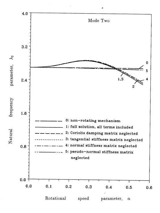
Figure 3.11: Natural frequency parameter vs. rotational speed parameter
