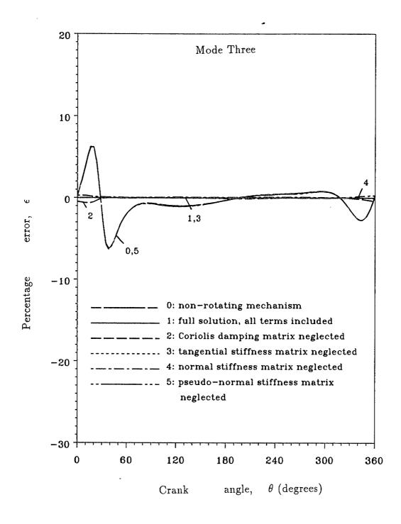
Figure 3.16: Percnetage error in natural frequency vs. crank angle,  $\Omega = 500$  rad/sec
