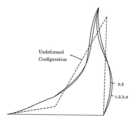
Figure 3.25: Forth mode shape,  $\theta=10^{\circ}, \Omega{=}1000~\rm{rad/sec}$
