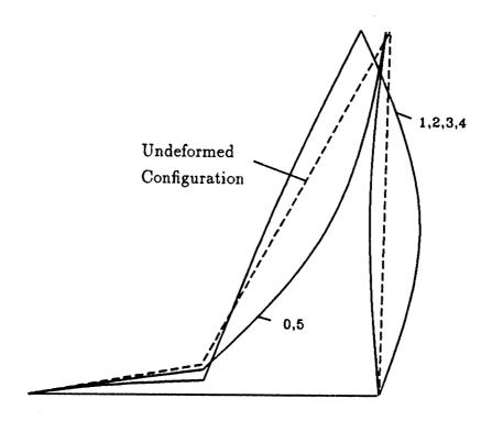
Figure 3.23: Second mode shape,  $\theta=10^{\circ}, \Omega=1000 \text{ rad/sec}$
