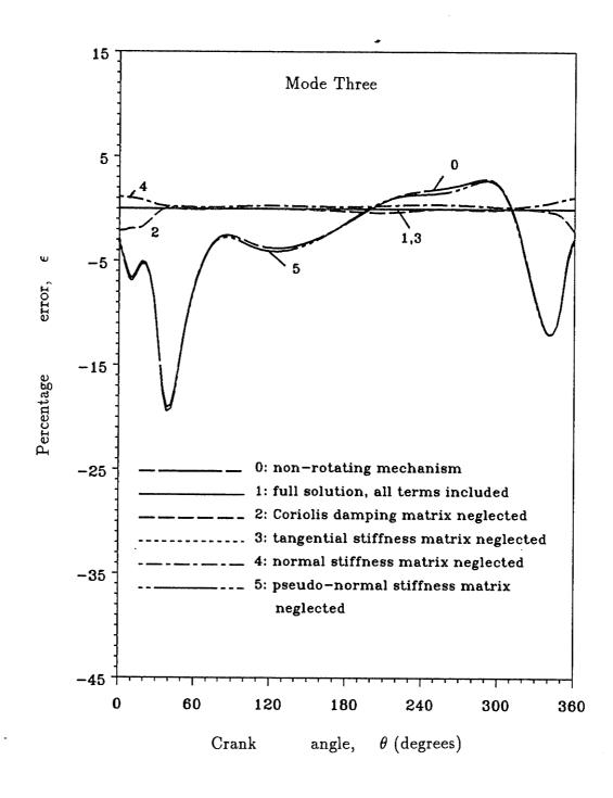
Figure 3.20: Percentage error in natural frequency vs. crank angle,  $\Omega$ =1000 rad/sec
