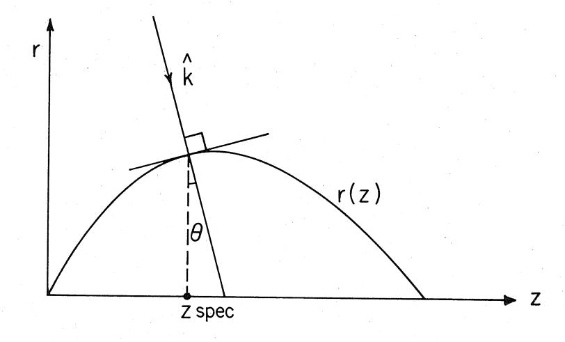
Fig. I.2 Geometric Optics inverse scattering geometry.
