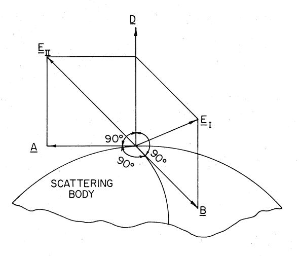
FIG. 2.1. Orthogonal Vector Triplet  $\underline{A}$ ,  $\underline{B}$ ,  $\underline{D}$  and Additional Vectors  $\underline{E}_{\underline{I}}$ ,  $\underline{E}_{\underline{I}}$
