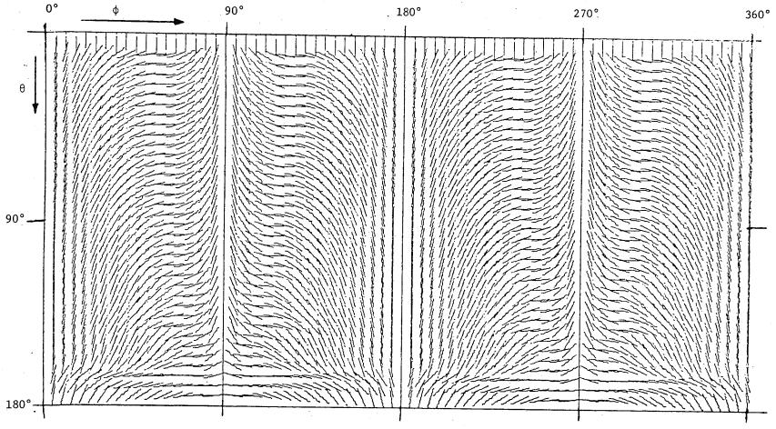
Fig.2.2a Vector  $\underline{A} = \underline{E}\underline{x}\underline{E}^* - \eta \eta^*\underline{H}\underline{x}\underline{H}^*$  plotted on the surface of a sphere of ka = 5,  $\eta = 0.5 /0^\circ$
