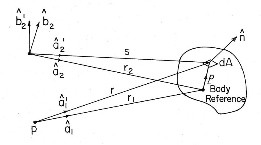
Fig. I.I Bistatic Symbols and Reference Directions.
