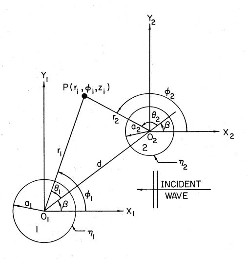
FIG. 4.2. SCATTERING BY TWO CYLINDERS OF RADII a\_1 AND a\_2 AND SURFACE IMPEDANCES  $\eta_1$  AND  $\eta_2$
