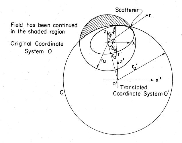
Fig.5.4. 3-D Analytic Continuation of the Electromagnetic Field on a  $\phi$  = Constant Plane using Outside Expansion.
