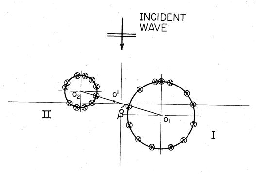
Fig. 4.10. Identification of Two Cylinders of Elec. Radii ka<sub>1</sub> = 2 , ka<sub>2</sub> = 1 ; Surface Impedances  $\eta_1$  = 0.1/30° ,  $\eta_2$  = 0.25/60° , Elec. Distance between the Centers kd = 5 ,  $\beta$  = 75°
