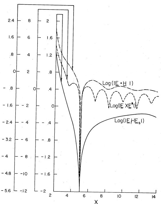
Fig. 4.5a Plot of Log { $|\underline{E} \times \underline{E}^*|^2$ }, Log{ $|\underline{E}_i| - |\underline{E}_s|$ }, Log{ $|\underline{E} \cdot \underline{H}|$ } Versus Radiant Vector X=kR for a Cylindrical Target of ka = 5.0,  $\eta$  = 0 for a Ray  $\phi$  = 22.5°
