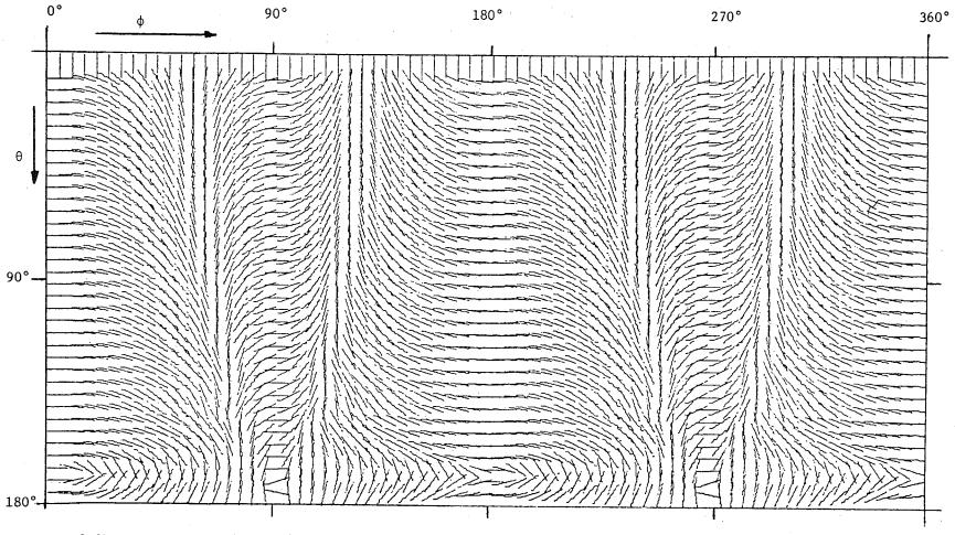
Fig.2.2b Vector  $\underline{B} = \eta \underline{E} * x \underline{H} - \eta * \underline{E} x \underline{H}$  plotted on the surface of a sphere of ka = 5,  $\eta = 0.5 / 0^{\circ}$
