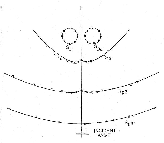
Fig. 5.6 b. Loci of Successive Minima of  $\underline{E} \times \underline{E}^*$  and  $\underline{E} \cdot \underline{H}$  for Two Pefectly Conducting Spheres of Elec. Radii  $ka_1 = ka_2 = 0.4$  and Separation between the Centers kd=1.2,  $\alpha=90^\circ$
