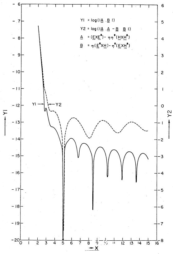
Fig. 5.8 c. Plot of YI and Y2 vs Radiant Vector X for a Spherical Target of ka=5.0,  $\eta$ = 0.433+j.25 for  $\theta$ =30°,  $\phi$ =90°
