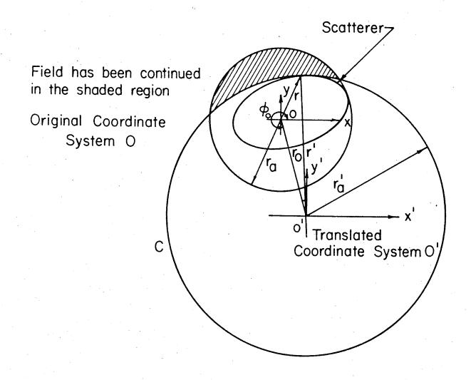
FIG.4.3. ANALYTIC CONTINUATION OF THE ELECTRO-MAGNETIC FIELD USING OUTSIDE EXPANSION
