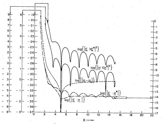
Fig. 5.7a. Plot of Log  $\{|\underline{H}_T \times \underline{H}_T^*|^2\}$ , Log  $|\underline{H}_i - \underline{H}_s|$ , Log  $(|\underline{E}_T \cdot \underline{H}_T|)$ , Log  $(|\underline{E}_T \cdot \underline{H}_T^*|)$ , Log  $(|\underline{E}_T \cdot \underline{H}_T^*|)$ , versus Radiant Vector X=kR for the Spherical Case ka=5.0,  $\eta = \omega$ ,  $\theta = 22.5$  and  $\phi = -90^{\circ}$
