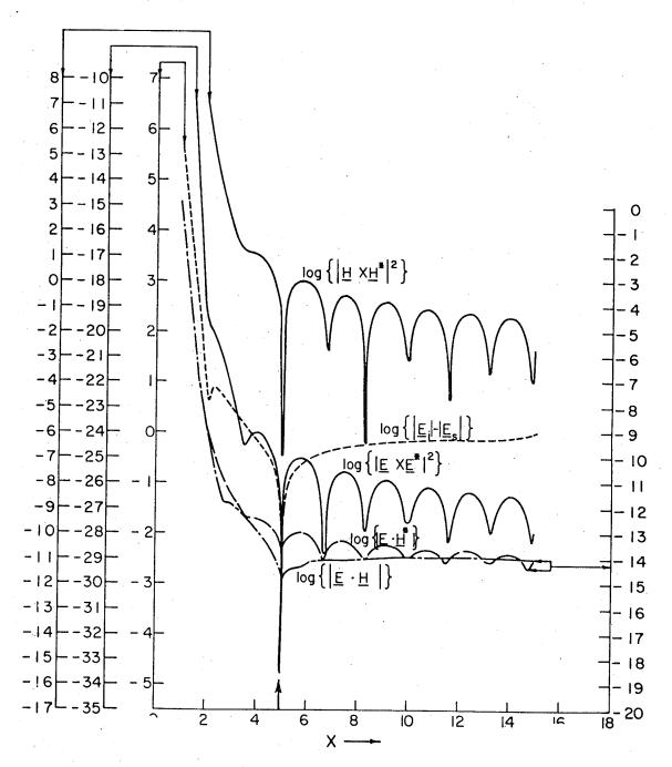
Fig. 5.5a. Plot of  $Log\{|\underline{E} \times \underline{E}^*|^2\}$ ,  $Log||\underline{E}_i| - |\underline{E}_s||$ ,  $Log\{|\underline{E} \cdot \underline{H}|\}$ ,  $Log||\underline{E} \cdot \underline{H}^*||^2\}$  versus Radiant Vector X=kR for the Sperical Test Case ka=5,  $\eta$  = 0,  $\theta$ =22.5°
