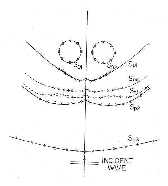
Fig. 5.12 Loci of Successive Minima of Yland Y2 for Two Conducting Spheres of Elec. Radii  $ka_1 = ka_2 = 0.4$  and Separation between Centers kd = 1.2,  $\alpha = 90^{\circ}$
