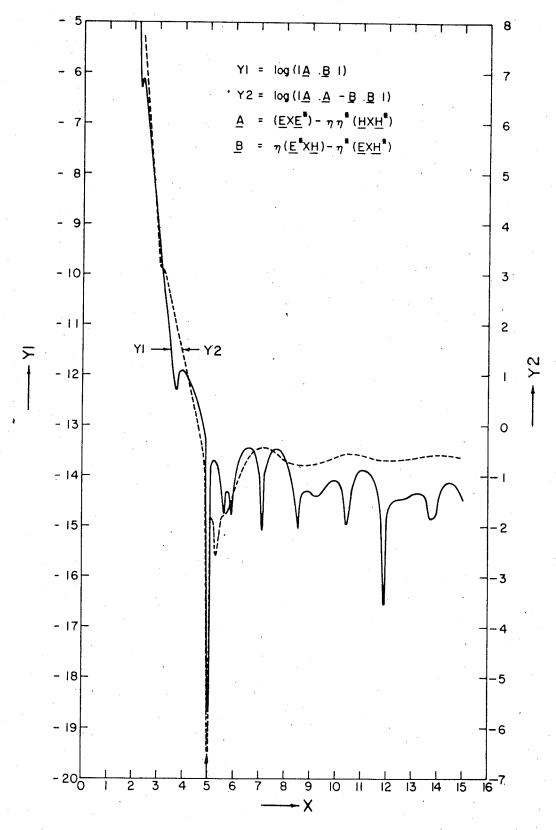
Fig. 5.8b. Plot of Y1 and Y2 vs Radiant Vector X for a Spherical Target of ka = 5.0,  $\eta = j(0.5)$  for  $\theta = 30^{\circ}$ ,  $\phi = 90^{\circ}$
