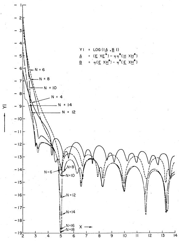
Fig. 6.2. Plot of YI vs Radiant Vector X=kR for the Spherical Test Case ka=5 for an increasing Number N of Expansion Terms  $\theta$ =22.5°,  $\phi$ =90°,  $\eta$ =2.0
