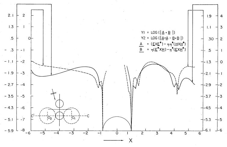
Fig.4.9a Plot of YI and Y2 vs Radiant Vector X for Two Cylinders of Elec. Radii  $ka_1 = 1$ ,  $ka_2 = 1$  and Separation Between Centers kd = 3 and the Surface Impedances  $\eta_1 = \eta_2 = 50 / 45^{\circ}$  along the Ray CC'.
