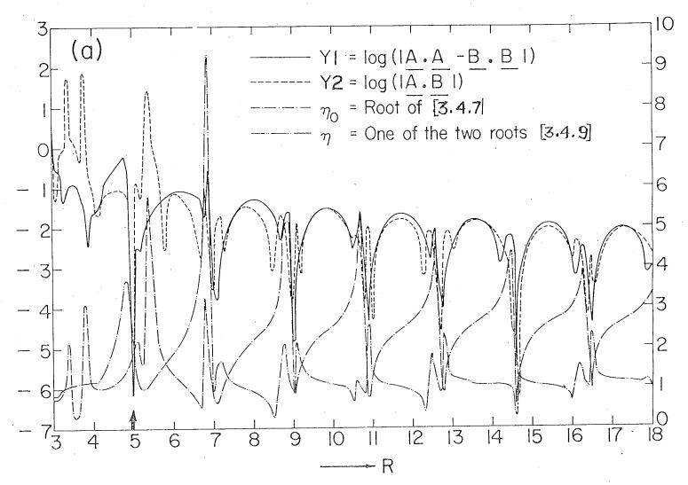
Fig. 5.13a . Plot of Y1 ,Y2,  $\eta_o$  and  $\eta_1$  vs Geometrical Distance R along a Ray ( $\theta$ =45°,  $\phi$ =60°) for a Spherical Target of a=5.0 , ka=5.0 and  $\eta$ =2.0
