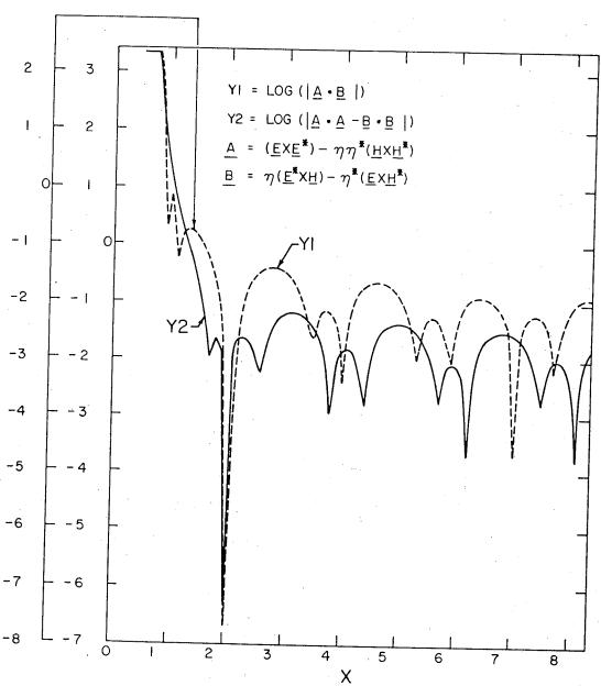
Fig.4.8a Plot of YI and Y2 vs Radiant Vector X for a Cylindrical Target of ka = 2 and  $\eta = 0.5 / 0^{\circ}$  along the Ray  $\phi = 45^{\circ}$
