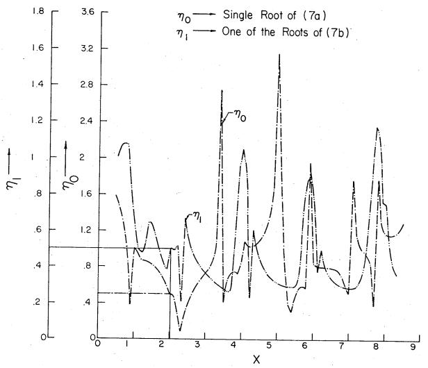
Fig.4.8c. Plot of  $\eta_0$  and  $\eta_1$  versus Radiant Vector X along a Ray ( $\phi$  = 45°) for a Cylindrical Target of ka = 2 and  $\eta$  = .5 $\underline{/0}$ °
