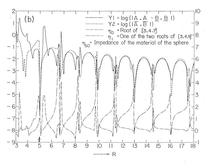
Fig. 5.13b Plot of Y1, Y2,  $\eta_o$  and  $\eta_1$  vs. Geometrical Distance R along a Ray ( $\theta$ =45°,  $\phi$ =60°) for a Spherical Target of a=5.0, ka=8.0 and  $\eta$ =2.0
