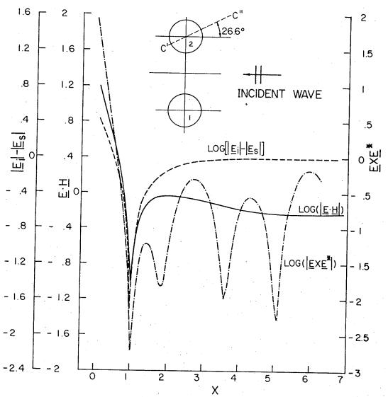
Fig. 4.7a. Plots of  $Log(I\underline{E}X\underline{E}^*I)$ ,  $Log[I\underline{E}_iI-I\underline{E}_sI]$  and  $Log(I\underline{E}\cdot\underline{H}I)$  for Two Perfectly Conducting Cylinders of Elec. Radii  $ka_1 = ka_2 = I$  Separation between Centers kd = 4 along the Ray C'C" of Fig. 6a
