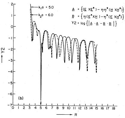
Fig. 5.9 b. Plot of Y2 vs Geometrical Distance R along a Ray  $(\theta$ =22.5, $\phi$ =90°) for a Spherical Test Case with Known  $\eta$ =2.0 and a=5.0 at Two Frequencie such that k a<sub>i</sub>=5.0 and k<sub>2</sub>=6.0
