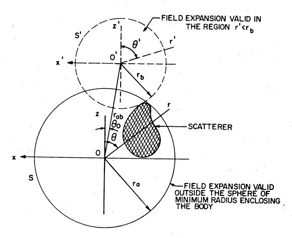
Fig.5.3. ANALYTIC CONTINUATION OF ELECTROMAGNETIC FIELD USING INSIDE EXPANSION ( $\phi$ =0°/ $\phi$ =180° PLANE)
