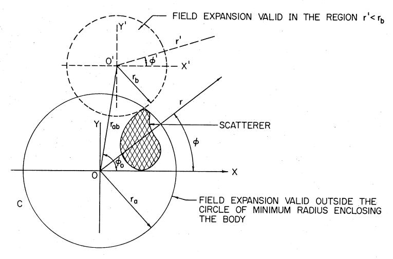
FIG.4.4. ANALYTIC CONTINUATION OF ELECTROMAGNETIC FIELD USING INSIDE EXPANSION
