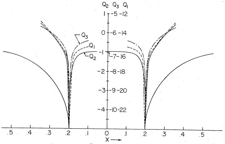
Fig. 5.6a Plots of  $Q_1 = \text{Log} |\underline{E} \times \underline{E}^*|^2$ ,  $Q_2 = \text{Log} [|\underline{E}_1| - |\underline{E}_S|]$  and  $Q_3 = \text{Log} [|\underline{E} \cdot \underline{H}|]$  vs Radiant Vector X for Perfectly Conducting Two-Sphere Configuration  $ka_1 = ka_2 = 0.4$ , kd = 1.2,  $\alpha = 90^\circ$  along the Ray  $\theta = 0$ ,  $180^\circ$  and  $\phi = 180^\circ$
