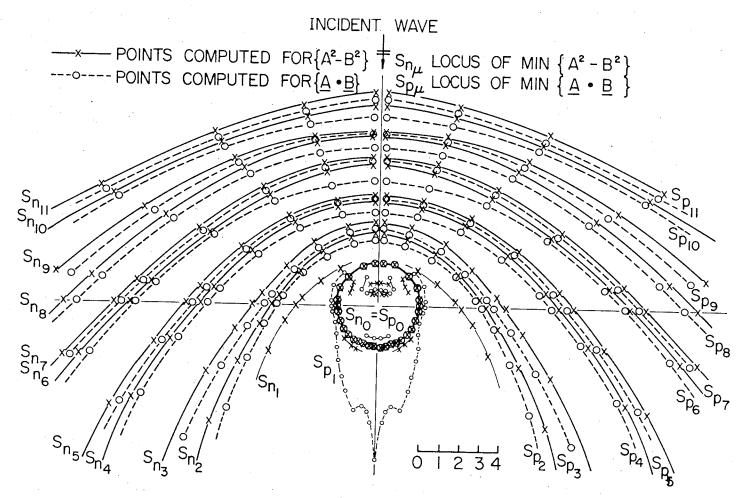
Fig.4.8b. Plot of the Loci  $S_{n\mu}$  and  $S_{p\mu}$  of Successive Minima of  $A^2$  -  $B^2$  and  $A \cdot B$  for a Cylindrical Target of Electrical Radius ka = 2 and Surface Impedance  $\eta$  = 0.5
