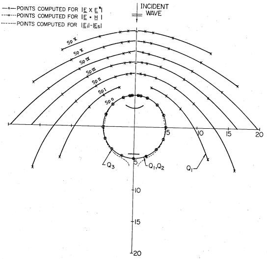
Fig. 4.5 b. LOCI OF SUCCESSIVE MINIMA OF <u>EXE</u>\* FOR A PERFECTLY CONDUCTING CYLINDER OF ELEC. RADIUS 5.0
