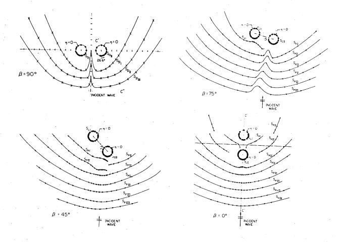
Fig. 4.6. Loci of Successive Minima of  $\underline{E} \times \underline{E}^*$  for Two Perfectly Conducting Cylinders of Elec. Radii  $ka_1 = ka_2 = 1.0$  and Separation between Centers kd = 4
