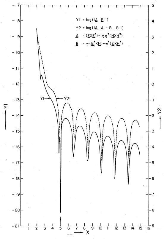
Fig. 5.8a. Plot of YI and Y2 vs Radiant Vector X for a Spherical Target of ka= 5.0 and  $\eta$  = 0.5 for  $\theta$  = 30.00,  $\phi$  = 90°
