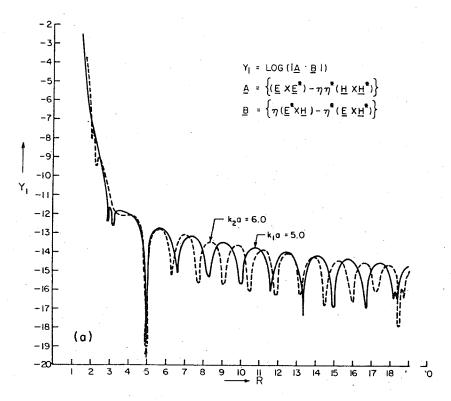
Fig. 5.9 a. Plot of YI vs Geometrical Distance R at Two Frequencies for a Sperical Test Case such that  $k_1a = 5.0$  and  $k_2a = 6.0$  for  $\eta = 2.0$ ,  $\theta = 22.5^{\circ}$  and  $\phi = 90^{\circ}$
