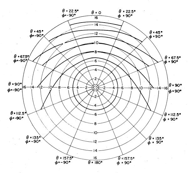
Fig. 5.5b. Surface Loci of Successive Minima of  $\underline{E}$  X  $\underline{E}^*$  for a Spherical Test case  $\eta$  =0 , ka = 5.0
