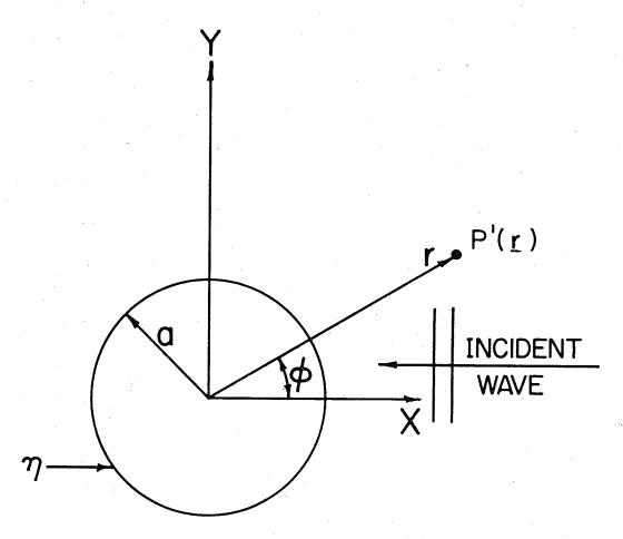
FIG. 4.1. A PLANE WAVE INCIDENT UPON A CYLINDER OF RADIUS  ${\bf a}$  AND SURFACE IMPEDANCE  ${\bf \eta}$
