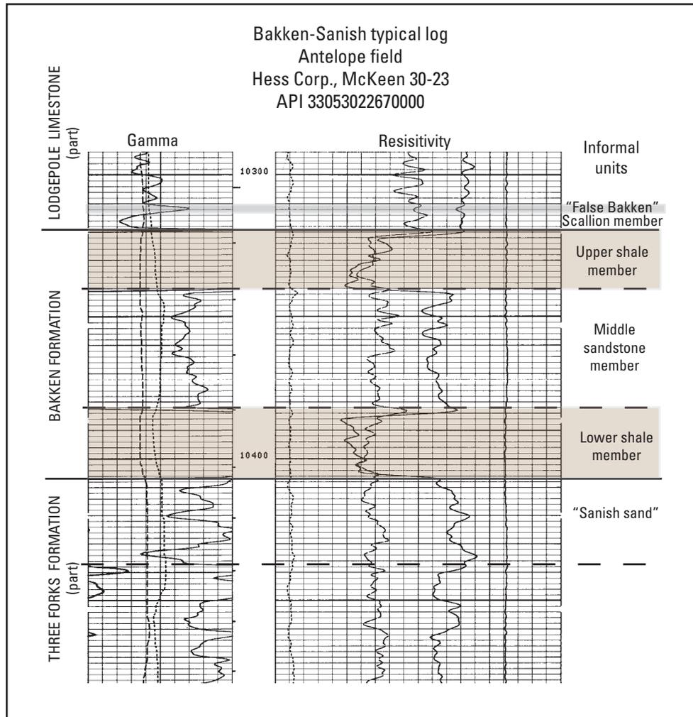
**Figure 6.** Typical gamma-ray (left) and resistivity (right) curves of the three informal members of the Devonian-Mississippian Bakken Formation, Sanish sand of the Devonian Three Forks Formation, and overlying Mississippian Lodgepole Limestone; location of well log is Antelope field, McKenzie County, N. Dak.
