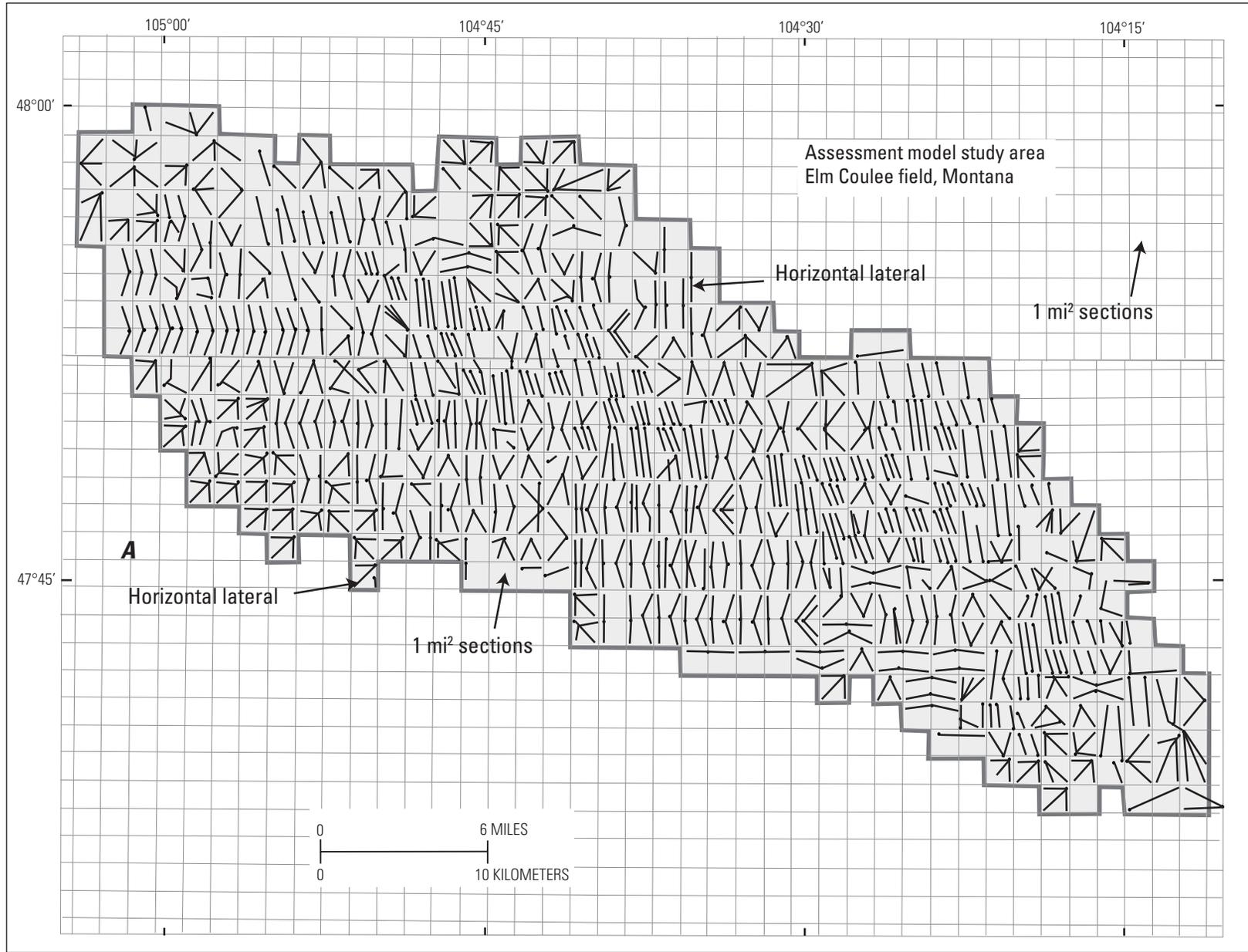
**Figure 18.** Well-bore configurations of horizontal laterals (bold lines) within 1-mi<sup>2</sup> (640-acre) sections used in effective drainage study area (shaded) at Elm Coulee field, Montana. Note direction and number of bold lines. Data and well-lateral configuration map from Montana Department of Natural Resources and Conservation (2008).
