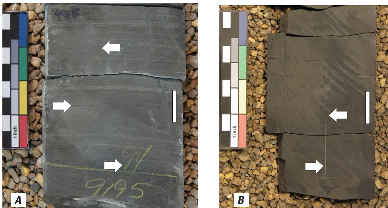
**Figure 9.** Photographs of microfractures in cores of the Bakken Formation, Parshall field, Montrail County, N. Dak. *A*, Horizontal microfractures (solid arrows) in lower shale member in the EOG Resources, Long 1-01H well. *B*, Vertical microfractures(?) in upper shale member in the EOG Resources, Inc., Fertile 1-12H well. Scale bars on right of photograph equal 1 in. Photographs courtesy of North Dakota Industrial Commission (2009).
