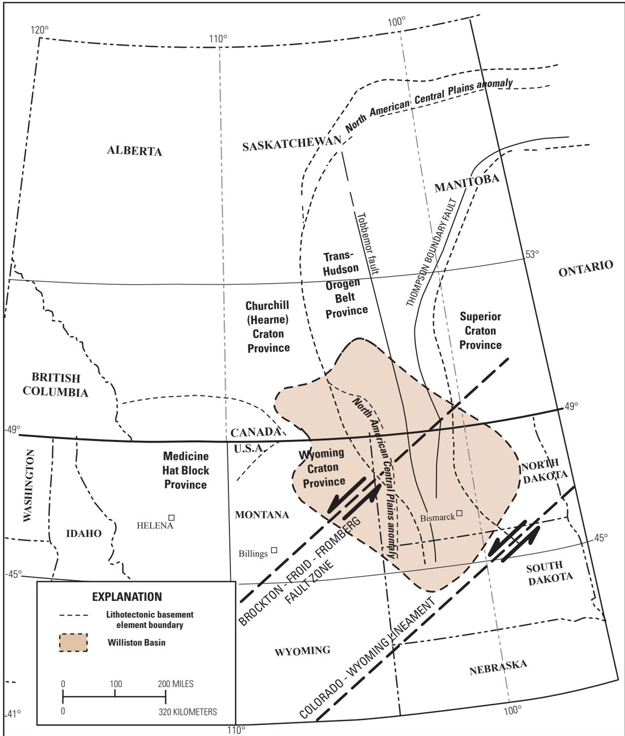
**Figure 1.** General extent of Williston Basin, two major fault systems responsible for the formation of the basin, and Precambrian basement structural provinces. Location of the North American Central Plains conductivity anomaly is also shown. Modified from Kent and Christopher (2007).
