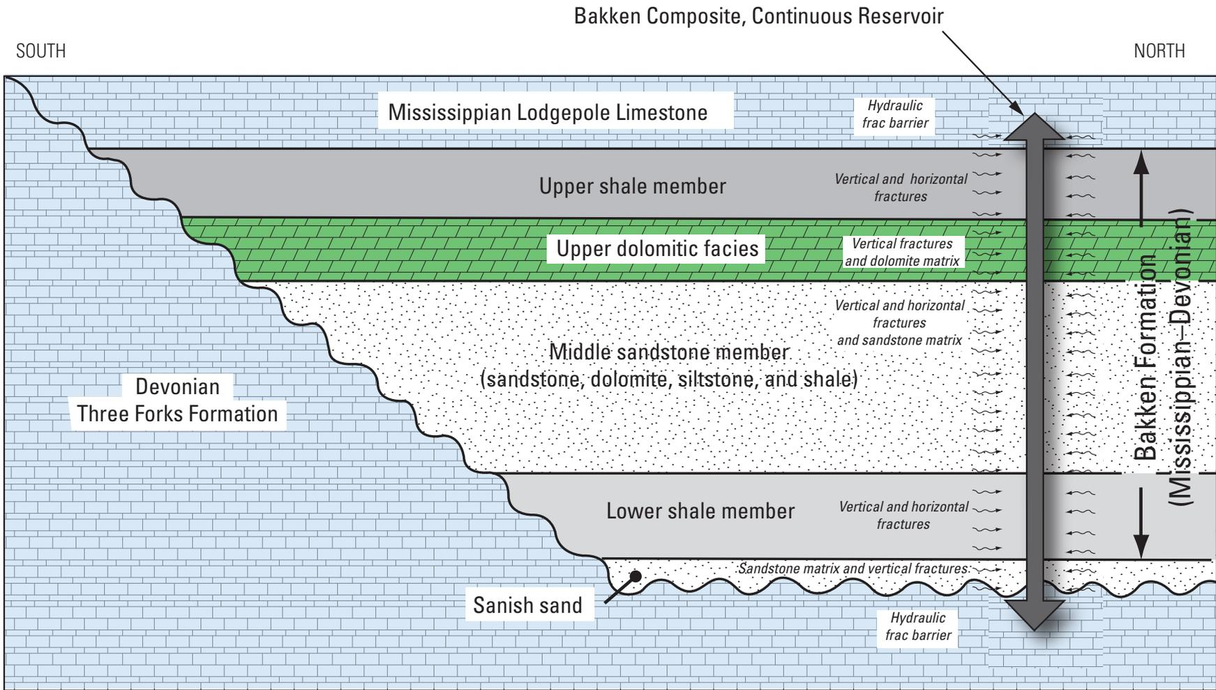
**Figure 7.** Schematic stratigraphic cross section from north to south across the depositional margin of the Devonian-Mississippian Bakken Formation, showing onlapping relation of members of the Bakken Formation, overlying and underlying units, and the Bakken composite continuous reservoir (large arrow). Physical properties related to oil production are also noted for each of the units. Sanish sand is informal member of Three Forks Formation. Modified from Pollastro and others (2008a).
