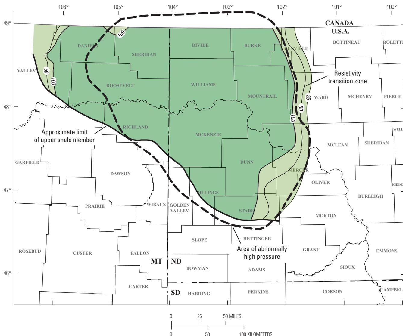
**Figure 10.** Log resistivity (in ohm-m) of upper shale member, Bakken Formation. Modified from Hester and Schmoker (1985). Area of abnormally high formation pressure (bold dashed line) approximated from Meissner (1984). Resistivity >100 ohm-m indicated by dark-shaded area; resistivity transition zone in lighter shaded areas between 25- and 100-ohm-m contours.
