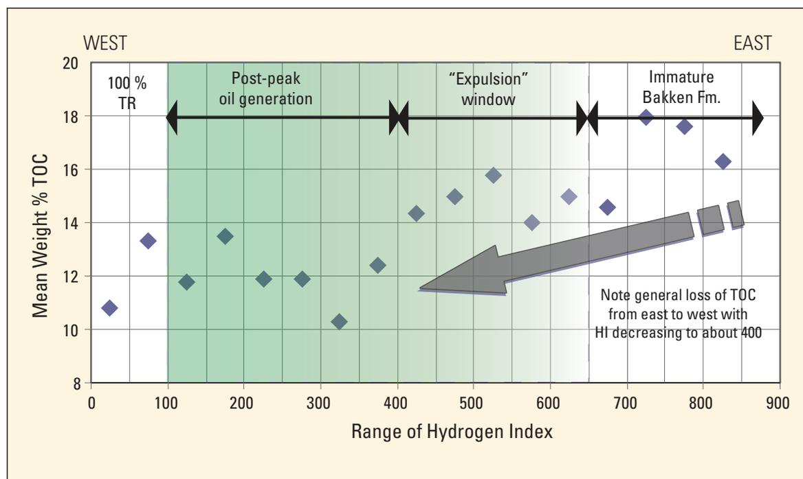
**Figure 14.** Plot of mean total organic content (TOC) versus range of hydrogen index (HI) in upper shale member of Bakken Formation, showing general decrease in TOC from east to west with decreasing HI and stages of oil generation with respect to HI. TR, transformation ratio (percent of hydrocarbons expelled).
