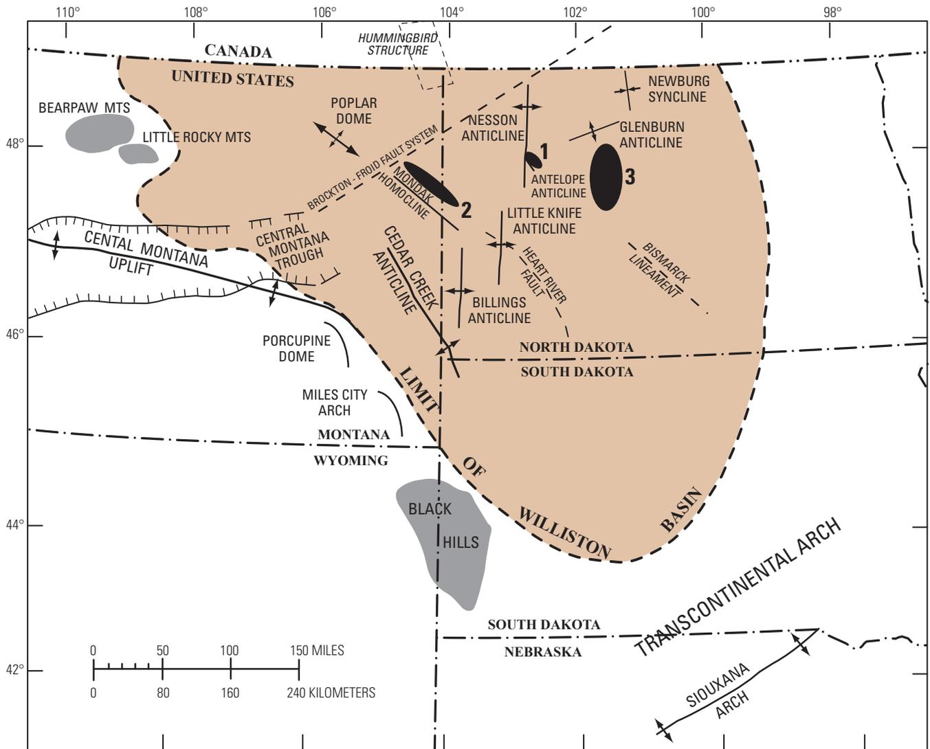
**Figure 2.** Present-day major structural elements of the U.S. portion of the Williston Basin. Solid black ovals show general location of three major areas of oil production from the Bakken Formation: Antelope field (1), Elm Coulee field (2), and Parshall and Sanish fields (3). Modified from Gerhard and others (1991).
