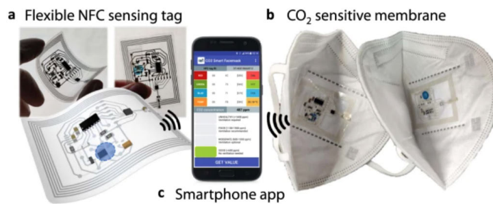
(b) Printed smart facemask. Reproduced from [32] under the terms of the Creative Commons Attribution (CC BY) License.
