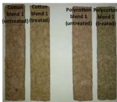
Figure 3.15. Treated and untreated bio-composite blends of cotton and polycotton for bending test
