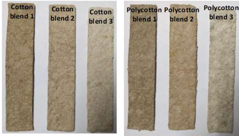
Figure 3.12 Treated bio-composite sheets for bending test
