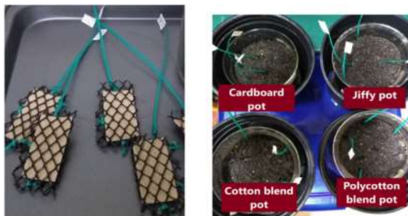
Figure 3.9. Soil burial test using different seedling pots
