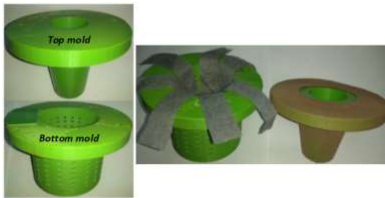
Figure 3.3. Mold used to form seedling pot
