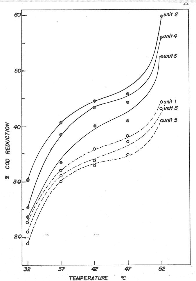
Fig. 3b. Percent COD reduction as a function of temperature in dairy cattle manure digestion. Solid lines indicate 15-day retention time; dotted lines indicate 10-day retention time. Units 1 and 2 have 0.15 lb.VS/ft<sup>3</sup>/day loading rate. Units 3 and 4 have 0.20 lb.VS/ft<sup>3</sup>/day loading rate. Units 5 and 6 have 0.25 lb.VS/ft<sup>3</sup>/day loading rate.
