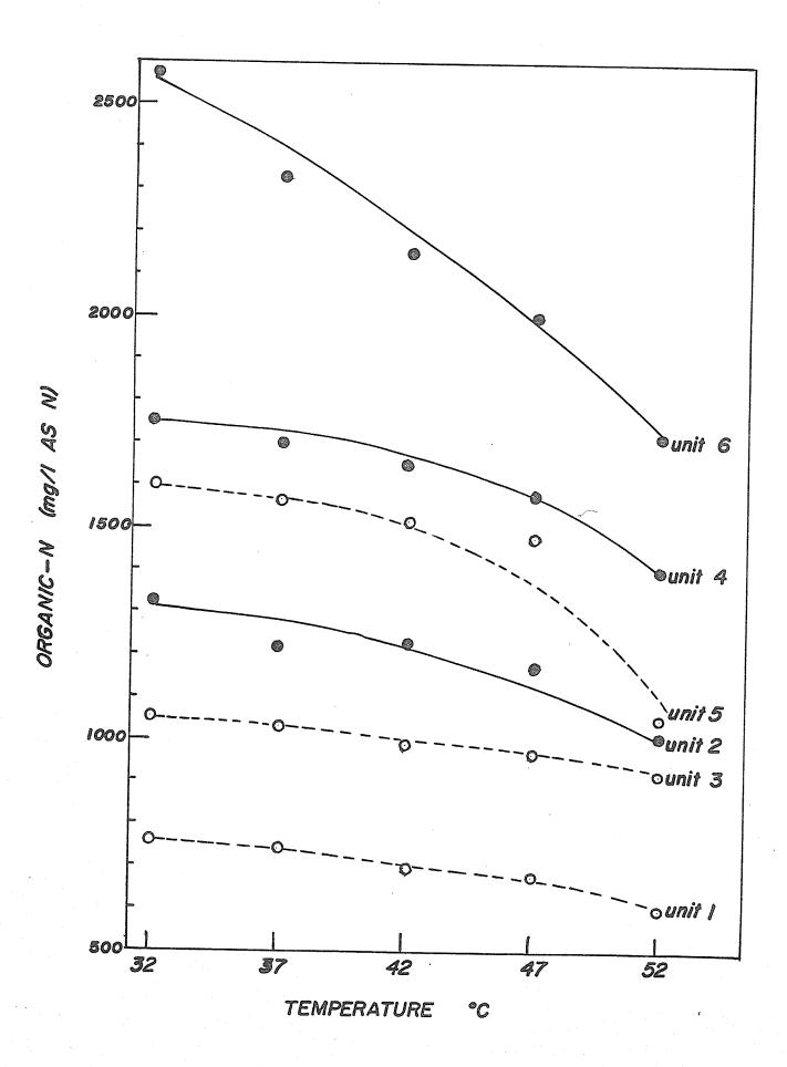
Fig. 8b. Organic-N concentration as a function of temperature in dairy cattle manure digestion. Solid lines indicate 15-day retention time; dotted lines indicate 10-day retention time. Units 1 and 2 have 0.15 lb.VS/ft<sup>3</sup>/day loading rate. Units 3 and 4 have 0.20 lb.VS/ft<sup>3</sup>/day loading rate. Units 5 and 6 have 0.25 lb.VS/ft<sup>3</sup>/day loading rate.
