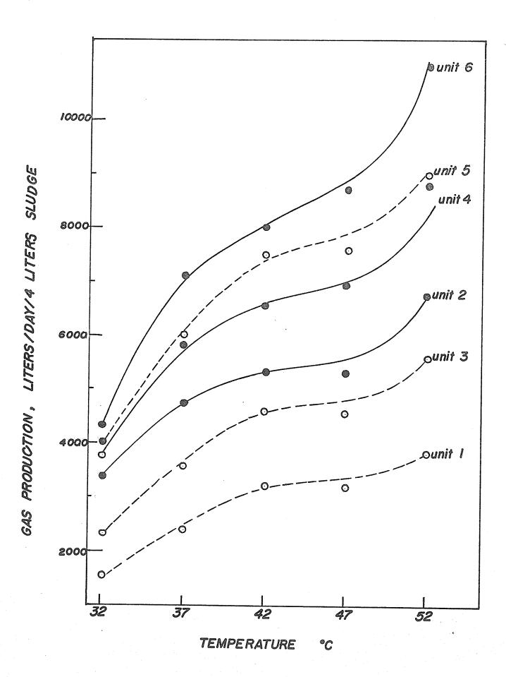
Fig. 11b. Gas production in litres/day/4 litre sludge as a function of temperature in dairy cattle manure digestion. Solid lines indicate 15-day retention time; dotted lines indicate 10-day retention time. Units 1 and 2 have 0.15 lb.VS/ft<sup>3</sup>/day loading rate. Units 3 and 4 have 0.20 lb.VS/ft<sup>3</sup>/day loading rate. Units 5 and 6 have 0.25 lb.VS/ft<sup>3</sup>/day loading rate.
