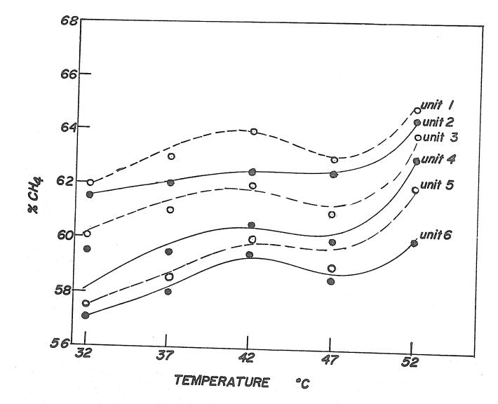
Fig. 10b. Percent methane as a function of temperature in dairy cattle manure digestion. Solid lines indicate 15-day retention time; dotted lines indicate 10day retention time.
