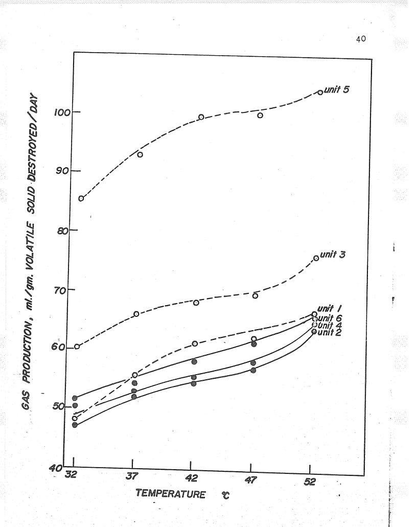
Fig. 9b. Gas production, ml./gm. VS destroyed/day as a
