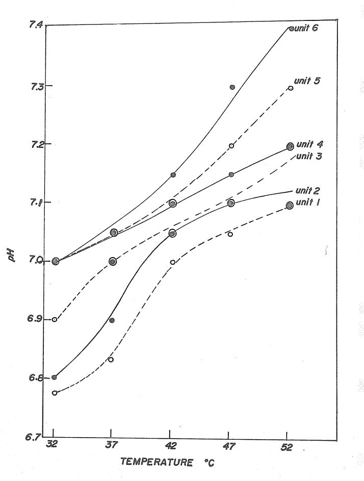
Fig. 5b. pH as a function of temperature in dairy cattle manure digestion. Solid lines indicate 15-day retention time; dotted lines indicate 10-day retention time. Units 1 and 2 have 0.15 lb.VS/ft<sup>3</sup>/day loading rate.
