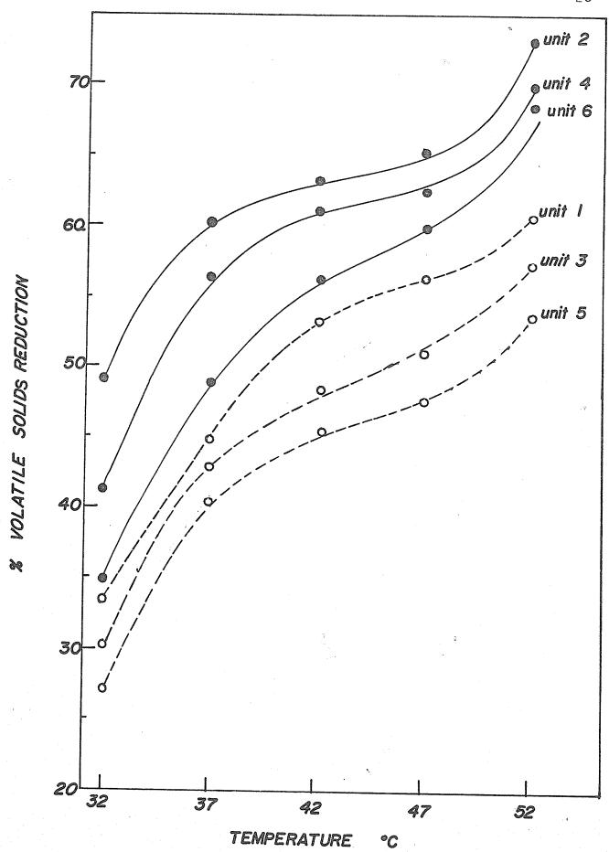
Fig. 2b. Percent volatile solids reduction as a function of temperature in dairy cattle manure digestion. Solid lines indicate 15-day retention time; dotted lines indicate 10-day retention time. Units 1 and 2 have 0.15 lb.VS/ft<sup>3</sup>/day loading rate. Units 3 and 4 have 0.20 lb.VS/ft<sup>3</sup>/day loading rate. Units 5 and 6 have 0.25 lb.VS/ft<sup>3</sup>/day loading rate.
