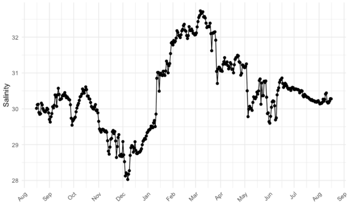
Figure S2.3 JB-M2 time series of daily average salinity values from August 2021 to August 2022. Measurements taken from CTD in 5 minute increments located on the mooring at a depth of ~41m.
