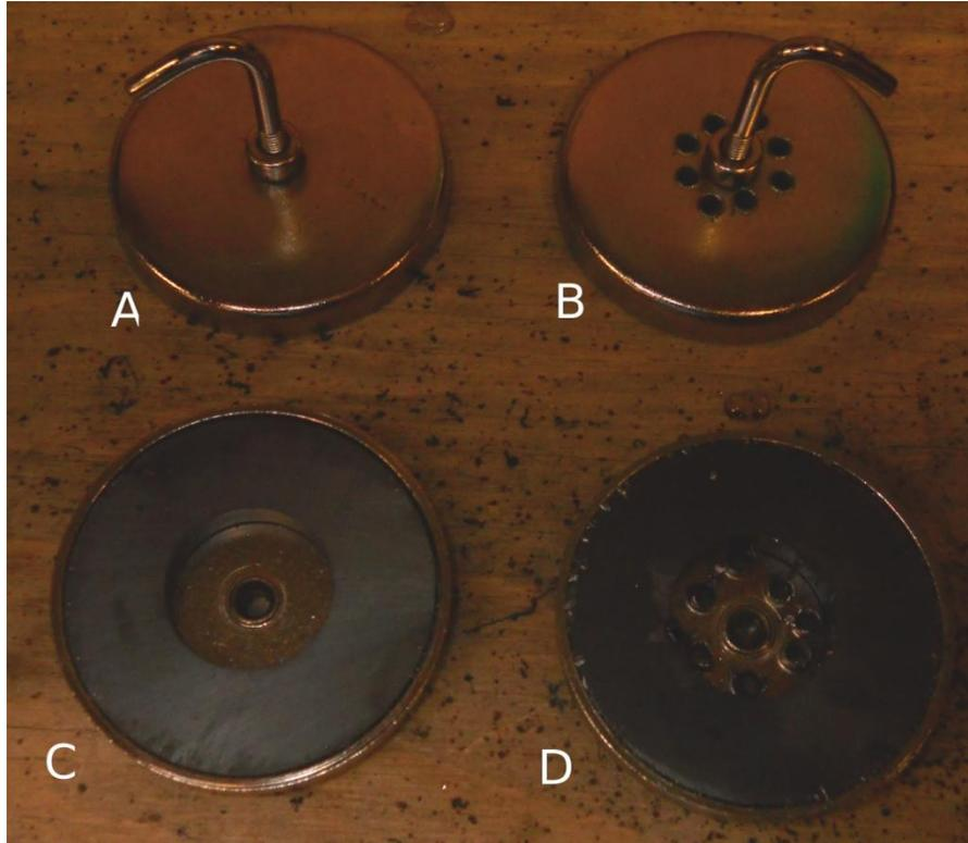
Figure 5.4. Filter retaining magnet detail. Left undrilled magnets. Right drilled magnets. A and B top view of magnet. C and B bottom view of magnet.
