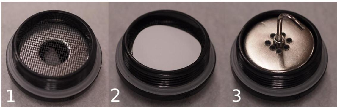
Figure 5.7 Filter setup. 1. Place screen on washer in filter support unit 2. Place filter on screen. Note: make sure not to contaminate the other filters with water from the sampling site. 3. Place magnet onto filter, screen, and washer. Press down to ensure that magnet is firmly seated.
