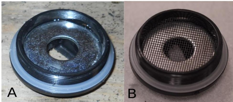
Figure 5.3. Filter support unit. A. Shows the retaining washer. B. Illustrates the filter support screen on the washer.
