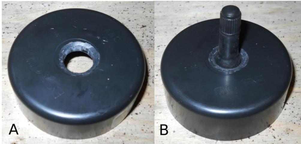
Figure 5.5 Valve installation. A. detail of hole for valve insertion. B. Valve inserted and glued in place.
