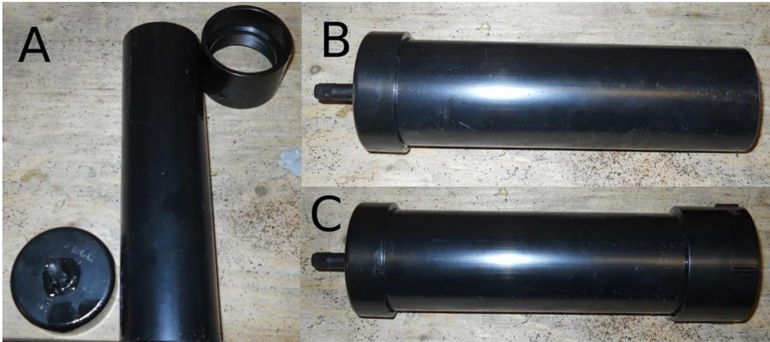
Figure 5.6 Assembly of the filter support unit. A. (From left to right) Valve cap, filter body tube, and female threaded cap adapter. B. Glue valve cap into place. C. Glue female threaded cap adapter into place.
