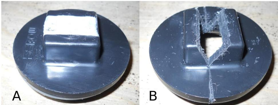
Figure 5.2. V Groove in filter support unit. A. ABS end cap. B. V-Groove cut in cap.
