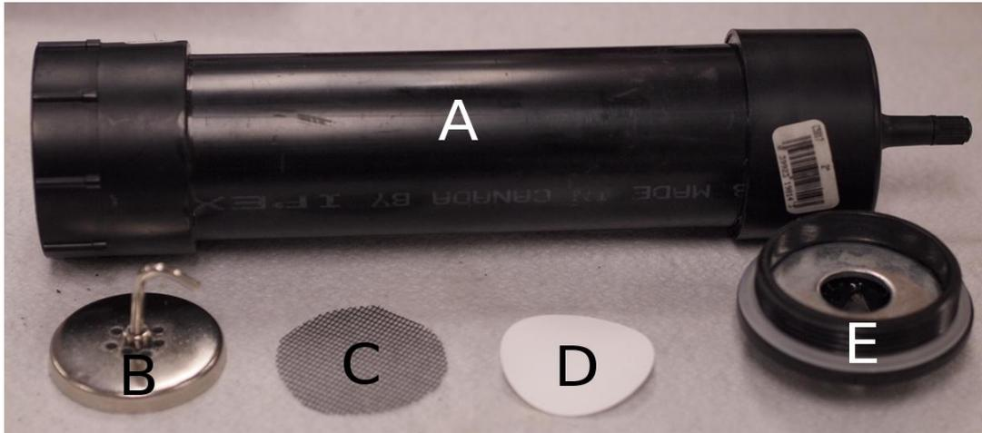
Figure 2.1. C.H.E.A.P. filtration unit. Filter body (A), filter support retaining magnet (B), filter support screen (C), membrane filter (D), and the filter support unit (E).
