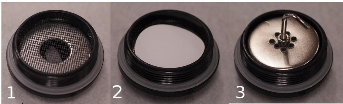
Figure 2.2 Filter support assembly. Screen was placed over the filter support unit (1) filter was then placed upon the filter support unit (2) the filter support retaining magnet was then pressed firmly into filter support system to ensure a proper seal (3).
