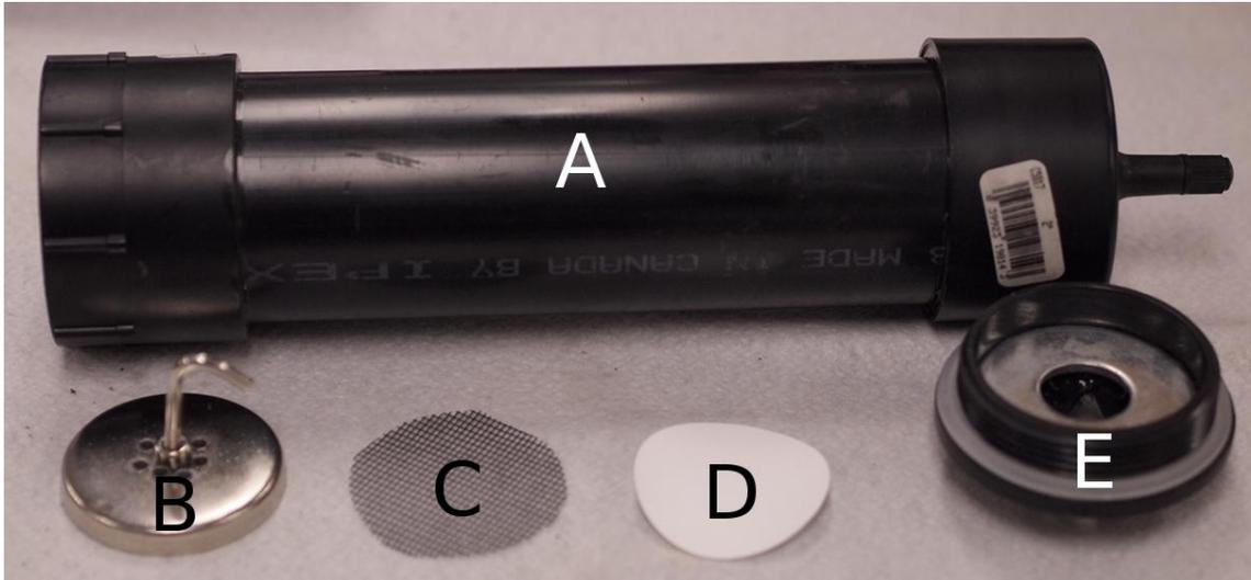
Figure 5.1. C.H.E.A.P. filtration unit components. A. Filter Body Unit. Calibrated for measured collection of water. Left side of the unit has a threaded receiver for Filter Support Unit. Right side has a tire valve for connection to bicycle pump to expel water. B. Filter support retaining magnet. C. Filter support screen. D. Membrane Filter. E. Filter support unit
