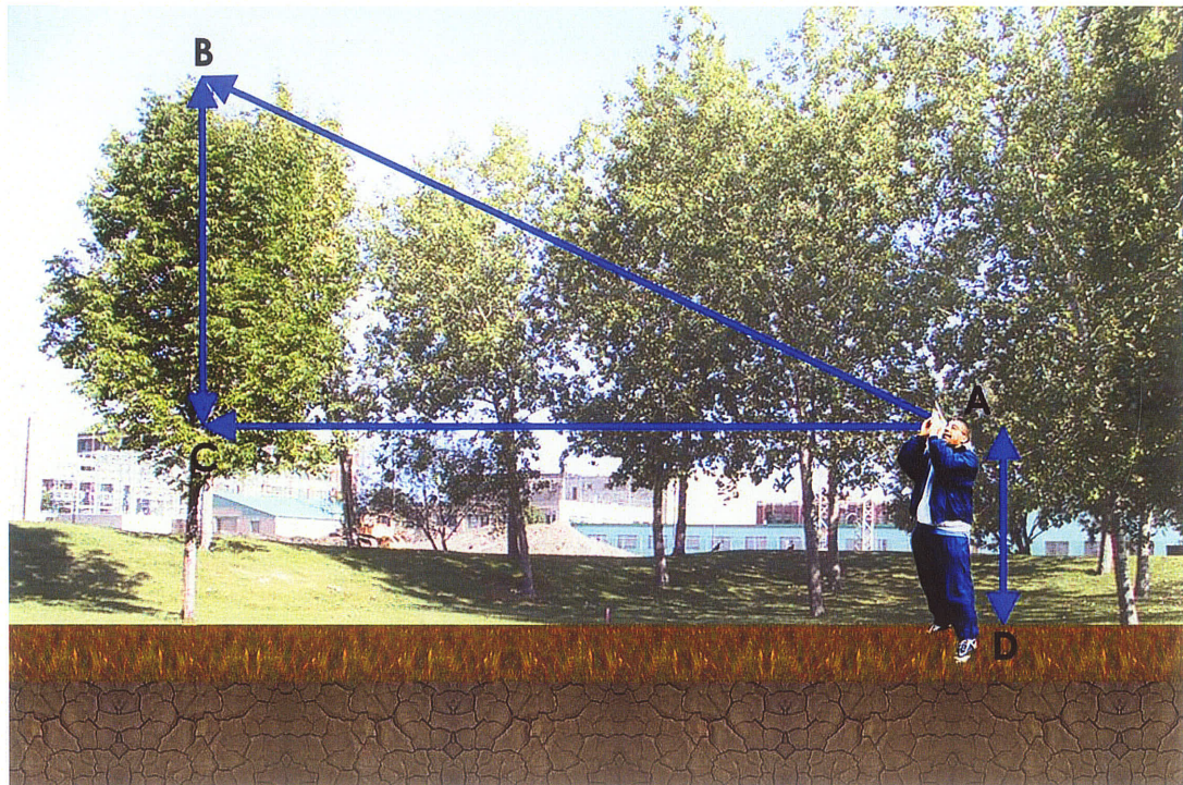
Figure 52. How to use a Clinometer. Photo by Author.
