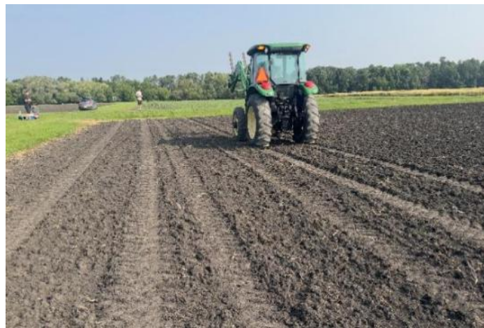
Figure 4.3. Compaction process with a John Deere tractor, showing wheel tracks where the soil cone index and bulk density measurements were taken.
